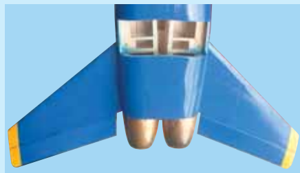
6B - Trial fit the horizontal stabilizers into the fuselage slots
