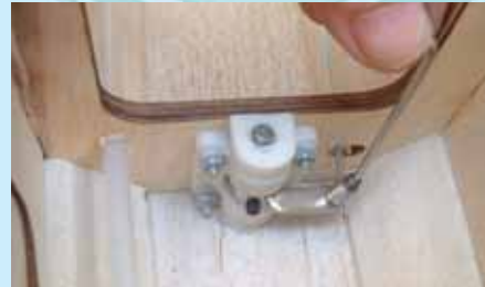
9H - Align and secure the EZ connector to the nose gear steering rod using the set screw.
