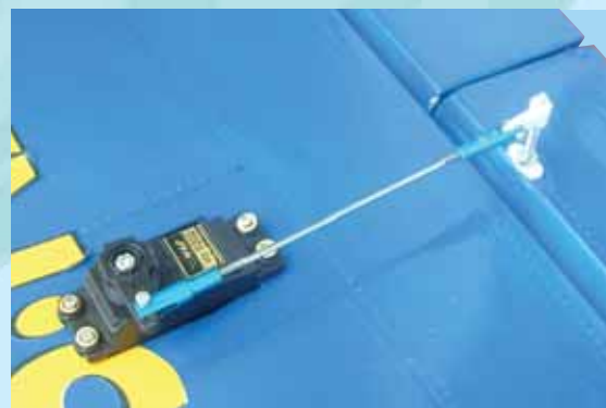
3C- Aileron control rod installed
