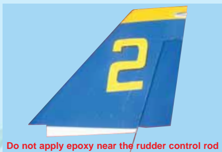
5E - Apply sufficient epoxy to both sides of the exposed wood
