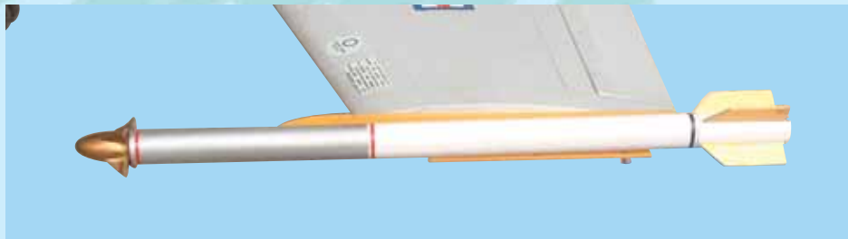
30E- Completed installation of dummy missile.
