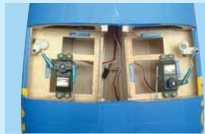
19C - With the servos and rudders at neutral, connect the clevises and then tighten the control horn set screws.
