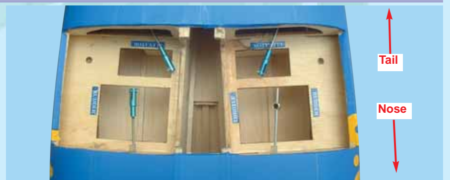
17A - Location of the 2 elevator, 2 rudder and throttle servos.
