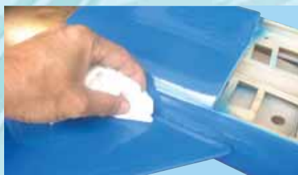
6E - Wipe off the excess epoxy
