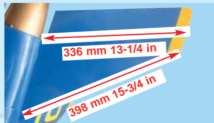
6D - Insert the left horizontal stabilizer into the fuselage and adjust the distance
