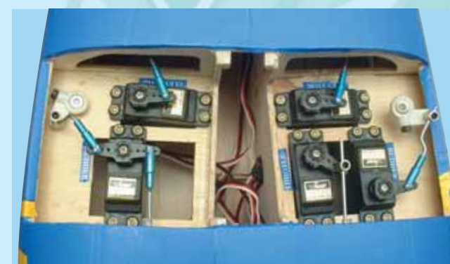
24A - Location of servos at aft end of fuselage
