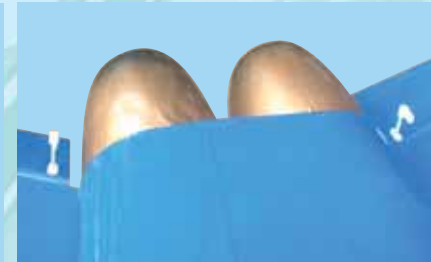
16C - Elevator control horns installed
