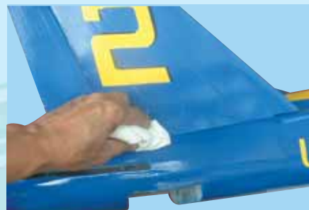
5F - Slide the vertical stabilizer into place. Wipe off any excess epoxy
