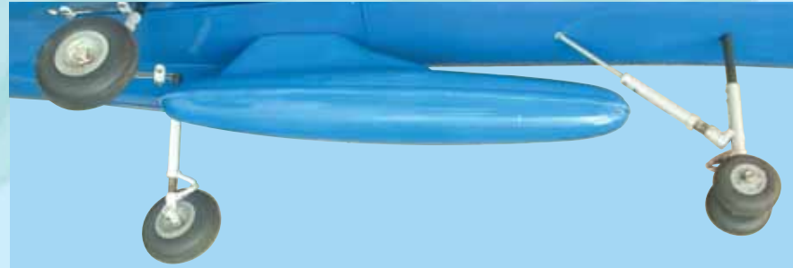
9I - Completed installation of the main and nose gear assemblies.
