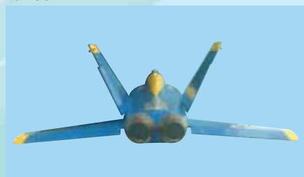
6F - Vertical and horizontal stabilizers installed.
