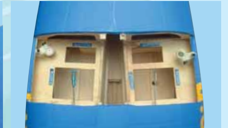
16D - Rudder control horns installed
