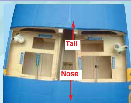
19A - Connect the 2 rudder control rods to the rudder control horns.
