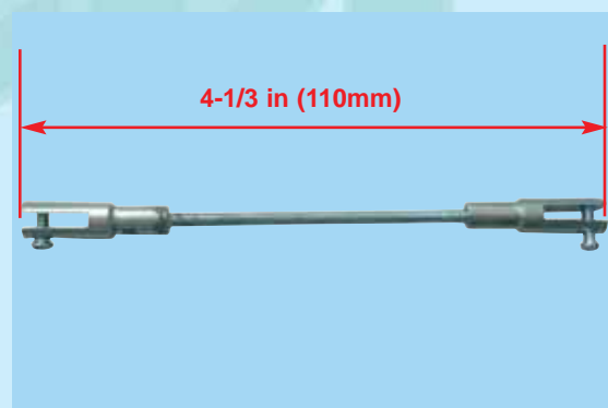
3A - Aileron control rod assembly
