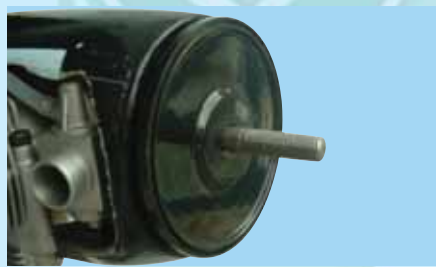
15B - Install the spinner backing plate
