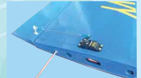
28C - Install the flap control rods between the servos and the horns.
