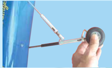
9E - Carefully pull the nose gear oleo strut out of the fuselage.
