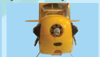
13D- Position the cowl over the mounting tabs. Note the strips are outboard. Align & center with respect to the motor shaft
