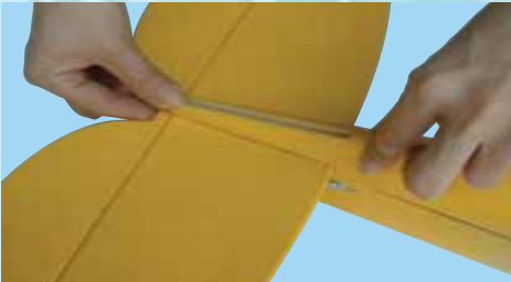
7J- Slide the horizontal stabilizer into place
