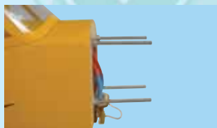
12J- Install four 3x50 [mm] bolt sets (supplied). Bolt-washer-former-washer-nut (front). Tighten the nuts securely & apply thread locker
