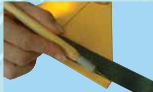
8C- Carefully cut through the covering. Do NOT cut the wood
