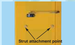
26B- Strut attachment point on the underside of the left wing
