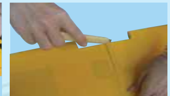
2F- Continue back around to the bottom of the wing & overlap the tape where you started. Trim off excess tape
