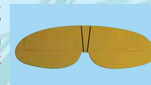
7C- Marked lines on horizontal stab
