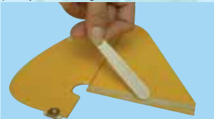
8E- Apply plenty of 30 minute epoxy
