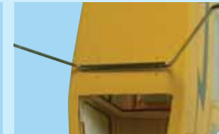
10C- Insert the pre-bent main landing gear into the fuselage
