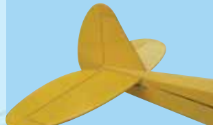
8A- Trial fit the vertical stabilizer into the fuselage slot
