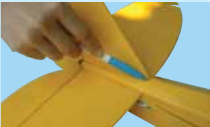
8B- Mark both sides of the vertical stabilizer
