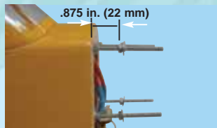
12K- Thread four 3 mm nuts onto the bolts as shown. The nuts should be all be evenly spaced at .875 in. (22 mm) from the firewall
