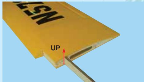
1C- Trial fit the wing joiner
