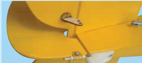
14C- Elevator control horn location
