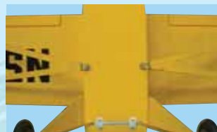
26F - Left & right struts attached to model.
