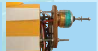
13B- Card stock strips overlying the cowl mounting tabs on the left and right side of the fuselage
