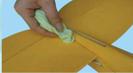
7K- Wipe off excess 30 minute epoxy
