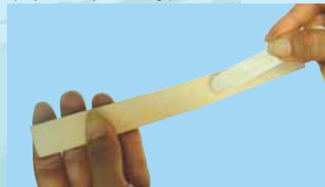
1D- Apply plenty of 30 minute epoxy to the wing joiner
