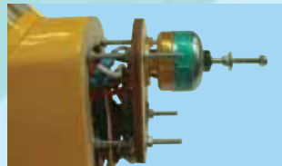
12L- Place four 3 mm washers on the bolts & then position the assembled power module. Secure in place with four more 3 mm washers & nuts. Tighten snugly
