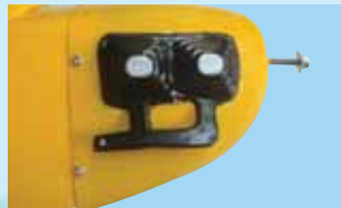
13F- Secure the cowl into place with four 2x10 [mm] screws
