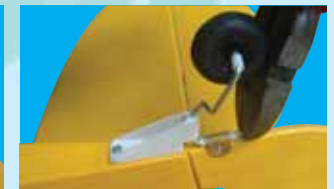
11D - Trim off the excess rudder steering wire.
