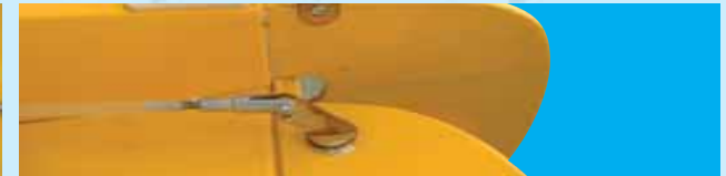
17B- Hold the elevator at neutral (not up, not down). Rotate the clevis to adjust the overall length. Then use the clevis screw to attach the clevis to the control horn. The clevis screw requires a 5/64 in. (2mm) hole. Secure the screw with thread lock
