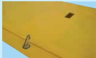
4B- Aileron control horn after installation using 30 minute epoxy
