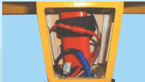
28C- Battery installed with security velcro
