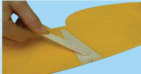
7I- Apply plenty of 30 minute epoxy to the horizontal stabilizer
