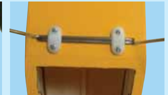
10D- Use two straps and four 10x2mm screws to mount the main landing gear assembly
