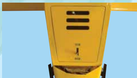
28D- Battery hatch installed with Fuse in place
