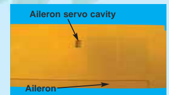
3B- Aileron servo location
