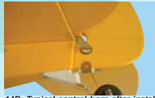
14B- Typical control horn after installation
