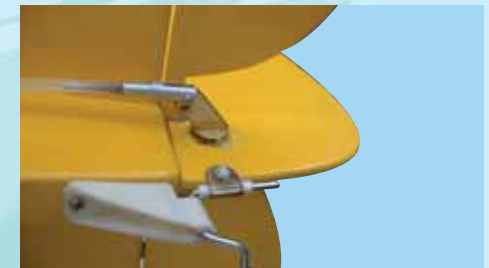
18A- Hold the rudder at neutral (not left, not right). Rotate the clevis to adjust the overall length. Then use the clevis screw to attach the clevis to the control horn. The clevis screw requires a 5/64 in. (2mm) hole. Secure the screw with thread lock
