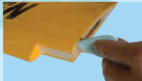
1F - Wipe off the excess epoxy then allow to cure
