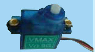
3A- Prepare the servos by fitting the rubber grommets & ferrules supplied with your servos
