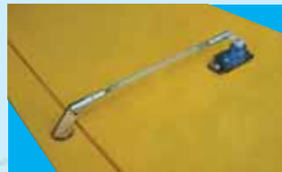
4C- Connect the aileron control rod between the servo arm and the control horn
