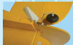
11B - Insert the rudder steering wire into the steering tube on the bottom of the rudder.
