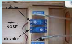
15C- Note the orientation and positions of the two servos in the servo tray
