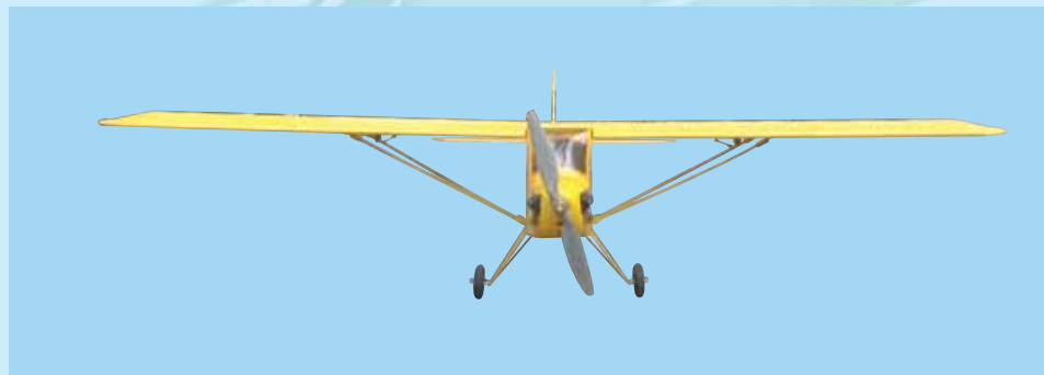
26G- Left & right struts attached to model
