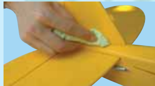
8F- Slide the stab into place & remove excess epoxy
