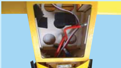
28B- Battery compartment as seen from bottom of fuselage
