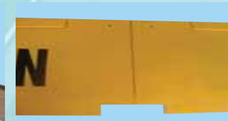
2B- Align the two wing panels and slowly close the gap until the wing root ends are firmly in contact with each other
