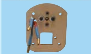
12D- Route the motor wire to the back of the firewall as shown
