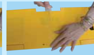
2E- Continue applying the tape over the top of the wing, pressing down firmly as you go
