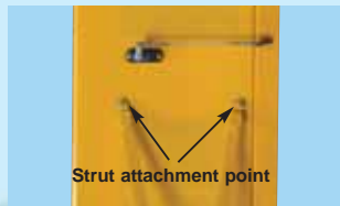
26E- Strut attached to the left wing panel
