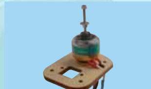
12C- Securely mount the aluminum motor backing plate to the firewall using 4, bolt & washer sets provided. Tighten the bolts securely and apply thread locker such as Pacer Z-42 (Blue)
