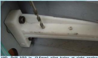
10D- Drill 3/32 in. (2.5mm) pilot holes at right angles through the beams
