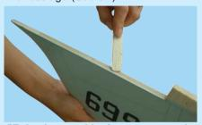
5F- Apply more 30 minute epoxy to the bottom of vertical stabilizer
