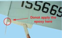
5E- Apply sufficient 30 minute epoxy to the lower stabilizer tonque. Avoid the control rod
