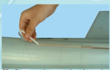
5D- Remove the covering from the fuselage
