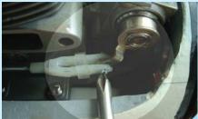
14A- Throttle control rod connected to the engine throttle arm
