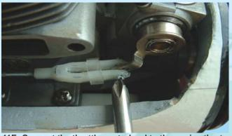
11E- Connect the throttle control rod to the engine throttle arm
