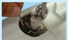
8C- Secure the steering arm to the nose gear wire by tightening the steering arm set screw
