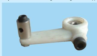
13A- Rudder control horn assembly
