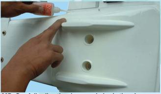
26D- Carefully align the clearance holes in the wing cover plate to ensure access to the wing bolts. Then use CA to attach the cover plate to the wing
