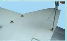
4B- Install the horizontal stabilizer onto the fuselage by using three 3-40 [mm] hex bolts and three wooden washer
