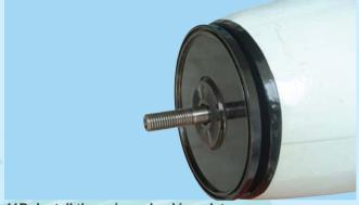
11B- Install the spinner backing plate
