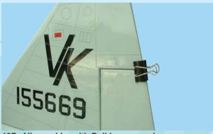
13B- Align rudder with Bulldog paper clamp
