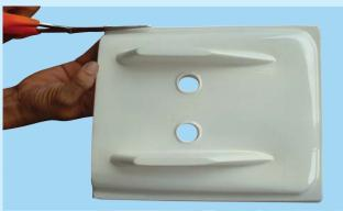
26B- Trim the wing cover plate using sharp scissors. See
