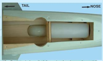
9D- Fuel tank installed into the fuselage after adding external fuel lines from tank forward to engine area
