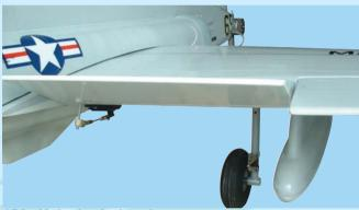
25G- Air brake deployed
