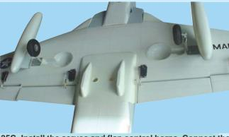
25C- Install the servos and flap control horns. Connect the flap control rods to the servo arms
