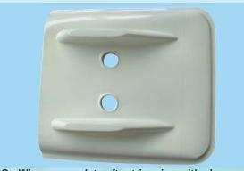
26C- Wing cover plate after trimming with sharp scissors
