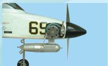
14C- Completed engine with throttle control connected and muffler installed
