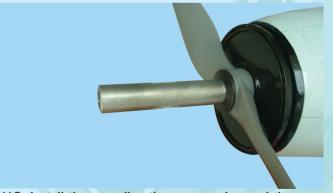
11C- Install the propeller, the prop washer and the prop nut
