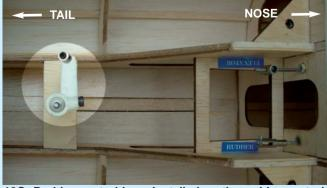
13C- Rudder control horn installed on the rudder control rod
