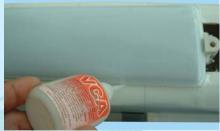
22C- Glue the nose gear cavity cover into place using CA glue
