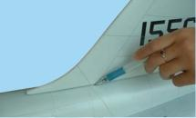
5B- Mark an outline around the area where the vertical stabilizer contacts the top of the fuselage
