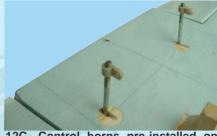
12C- Control horns pre-installed on the elevator torque rods
