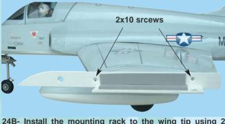
24B- Install the mounting rack to the wing tip using 2 screws 2x10 [mm]
