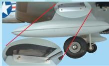
23D- Mount the dummy tanks to the aluminum rails on the wings
