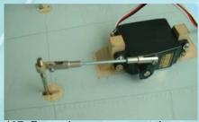
12E- For each servo, connect the control rod between the servo arm and the control horn
