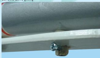
24D- Secure the missile to the mounting rack by using 2 screws, 1 in the top...
