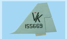
3B- Vertical stabilizer with preinstalled rudder and torque rod
