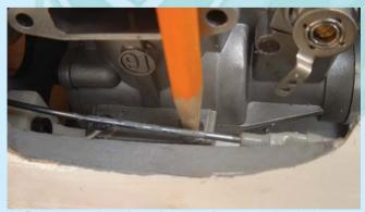
10C- Mark the location of the engine mounting holes
