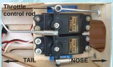
14B- The throttle servo controls the engine throttle using the throttle control rod
