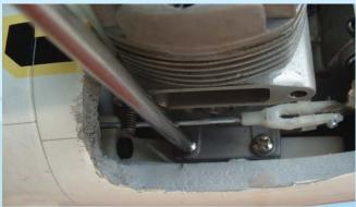
11F- Attach the engine to beams using four screws (supplied)
