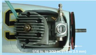
10B- Allow for a gap between the spinner back plate and the fuselage
