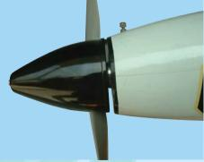
11D- Install the spinner cone using the retaining screw. Ensure the retaining screw is tight and secure
