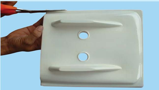
26B- Trim the wing cover plate using sharp scissors. See 26C
