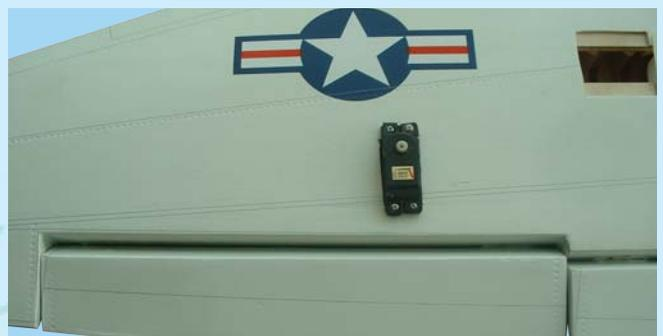
1C- Mount the aileron servos into the wing
