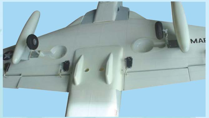
25C- Install the servos and flap control horns. Connect the flap control rods to the servo arms
