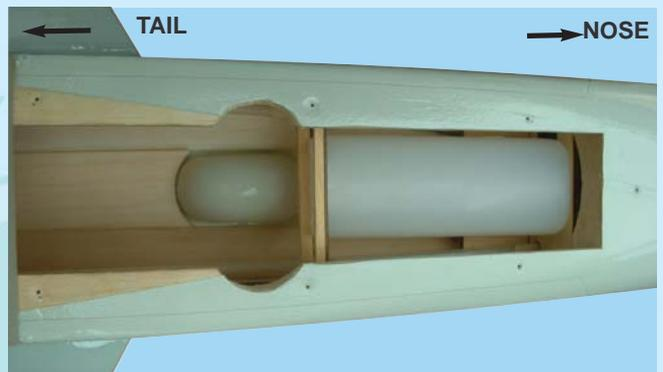
9D- Fuel tank installed into the fuselage after adding external fuel lines from tank forward to engine area
