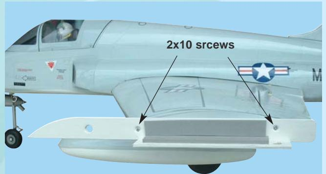
24B- Install the mounting rack to the wing tip using 2 screws 2x10 [mm]
