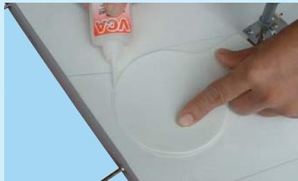
22B- Glue the main gear cavity covers into place using CA glue
