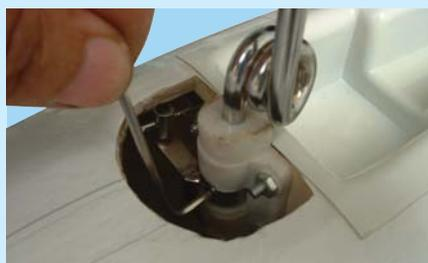
8C- Secure the steering arm to the nose gear wire by tightening the steering arm set screw
