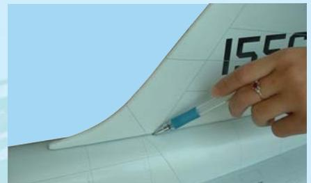
5B- Mark an outline around the area where the vertical stabilizer contacts the top of the fuselage
