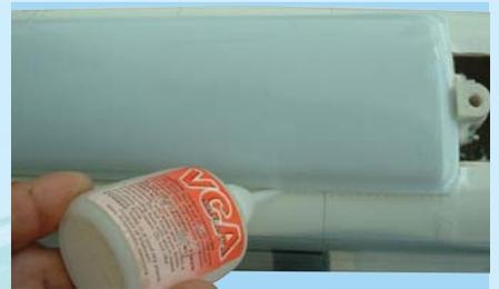
22C- Glue the nose gear cavity cover into place using CA glue
