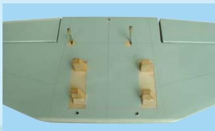
12B- Pre-installed elevator torque rods & servo rails
