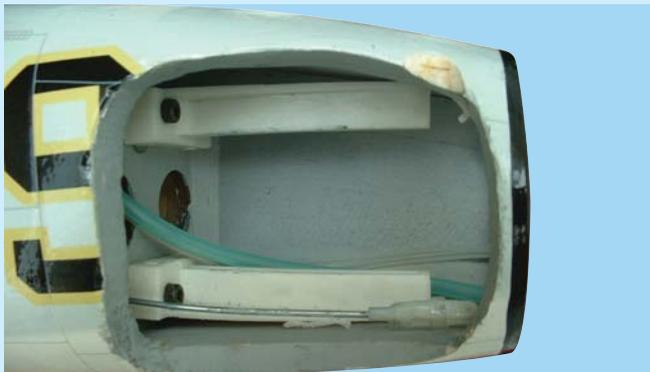
10A- Pre-installed engine mount
