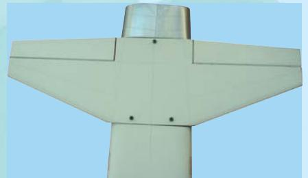
4C- Horizontal stabilizer attached to the fuselage
