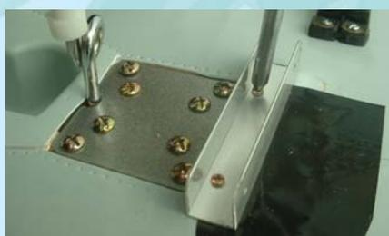
23C- Mount the mounting rails to the wing
