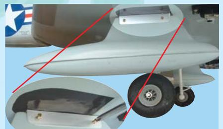
23D- Mount the dummy tanks to the aluminum rails on the wings
