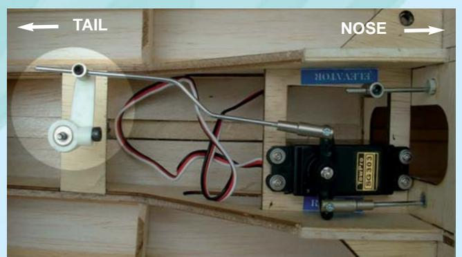
13D- Rudder control rod installed between the rudder servo and rudder control arm. Nose gear steering rod connected to opposite side of servo arm
