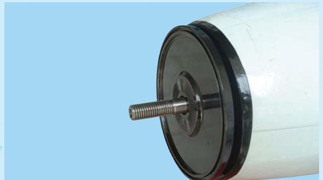
11B- Install the spinner backing plate
