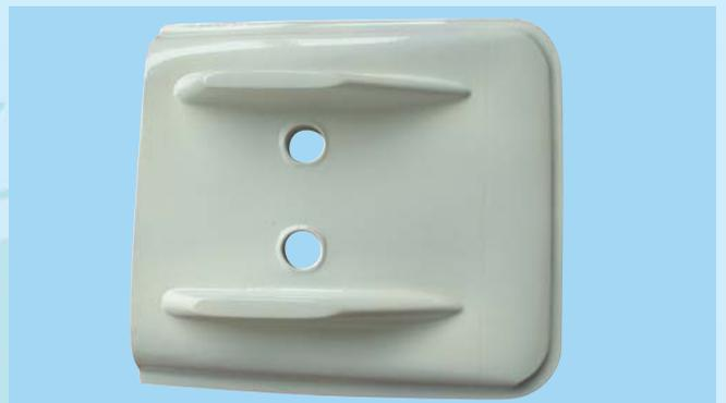
26C- Wing cover plate after trimming with sharp scissors
