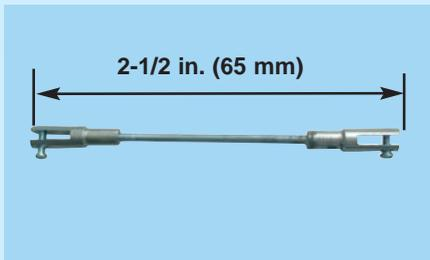
12A- Elevator control rod assembly
