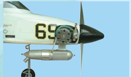
14C- Completed engine with throttle control connected and muffler installed
