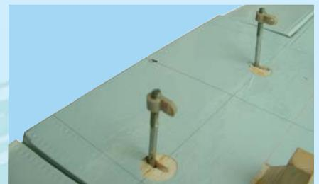
12C- Control horns pre-installed on the elevator torque rods
