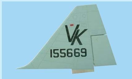
3B- Vertical stabilizer with pre-installed rudder and torque rod
