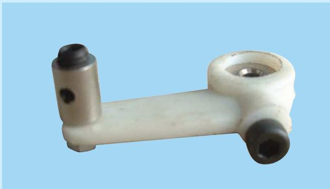
13A- Rudder control horn assembly
