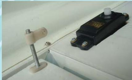
2B- Aileron control horn installed
