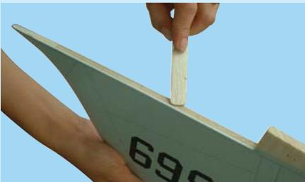
5F- Apply more 30 minute epoxy to the bottom of vertical stabilizer
