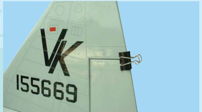
13B- Align rudder with Bulldog paper clamp
