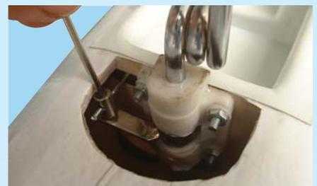
8D- Secure the EZ-connector to the nose gear push rod by tightening the EZ-connector set screw
