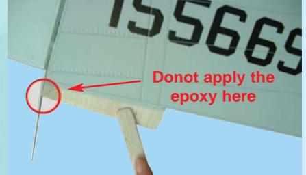
5E- Apply sufficient 30 minute epoxy to the lower stabilizer tongue. Avoid the control rod
