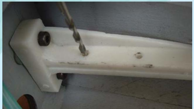
10D- Drill 3/32 in. (2.5mm) pilot holes at right angles through the beams
