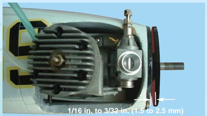
10B- Allow for a gap between the spinner back plate and the fuselage
