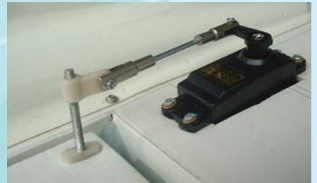
2C- Aileron control rod installed
