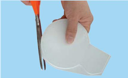
22A- Cut out the cavity covers using sharp scissors
