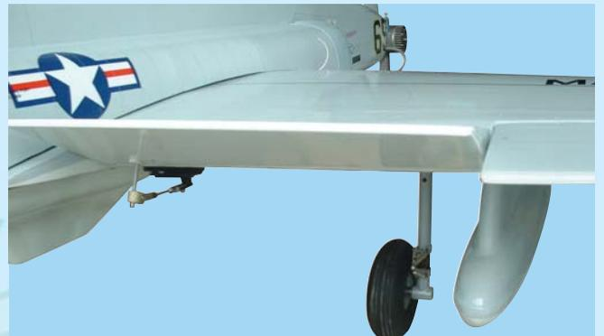
25G- Air brake deployed
