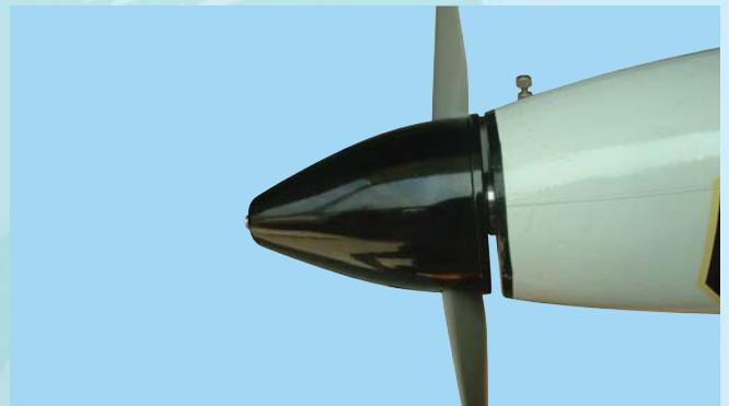
11D- Install the spinner cone using the retaining screw. Ensure the retaining screw is tight and secure
