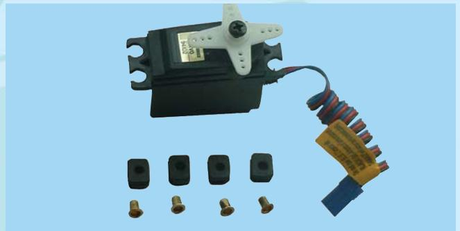
1A- Prepare the servos by fitting the rubber grommets & ferrules supplied with your servos
