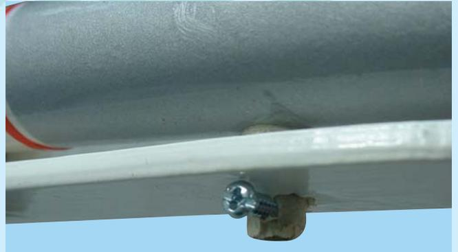
24D- Secure the missile to the mounting rack by using 2 screws, 1 in the top...
