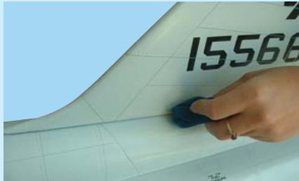
5G- Carefully press the vertical stabilizer into place and remove any excess epoxy
