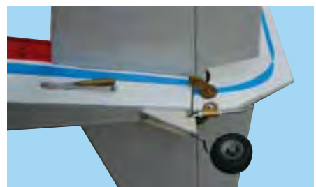
13F - Rudder control horn installed at correct location using 30 minute epoxy and retaining screw.
