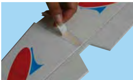
6E - Remove the covering from top surface
