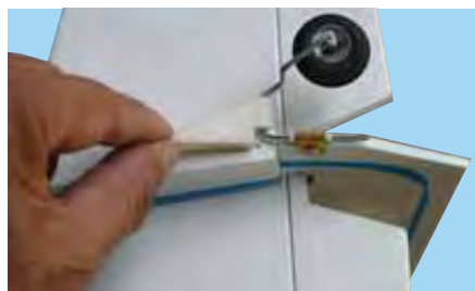
10C - Insert the tail wheel wire into the rudder sleeve tube.
