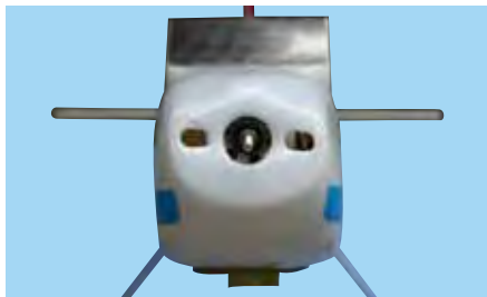
12B - Position the cowl over the mounting tabs. Align and center with respect to the motor shaft.
