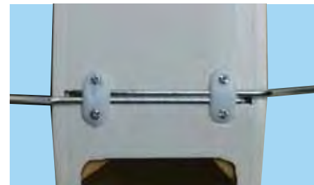
9D - Use two straps and four 10x2 [mm] screws to mount main landing gear assembly to the fuselage
