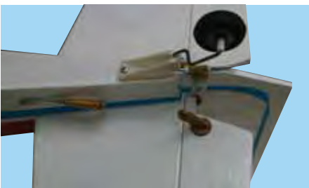
13D - Elevator control horn installed at correct location using 30 minute epoxy and retaining screw.
