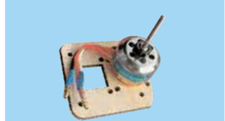
11C - Install the motor to the firewall using 4 bolts (3x10mm) & washer sets provided. Place washer on bolt and insert bolt through back of firewall & screw into tapped holes in motor mounting plate. Secure bolts with medium thread locker
