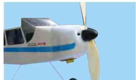
12D - With the BATTERY & FUSE REMOVED securely install the propeller
