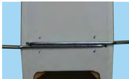
9C - Insert the pre-bent main landing gear into the fuselage
