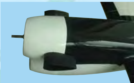
10H- Use CA glue to attach the dummy exhaust stacks to the cowl.
