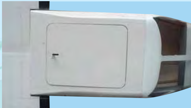
20D- Battery hatch installed
