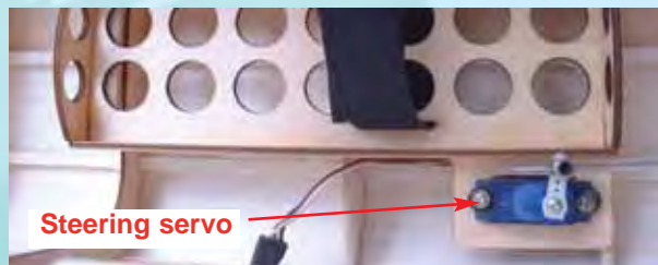
21.2 Nose steering rod connect to the nose steering servo arm
