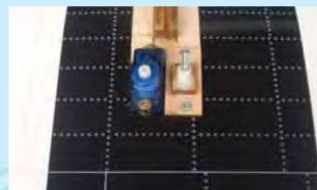
22C- Wing strut anchor installed in the left wing
