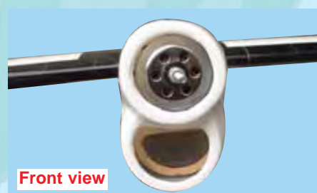
10D- Position the cowl over the engine covers. Align cowl & center about the motor shaft.
