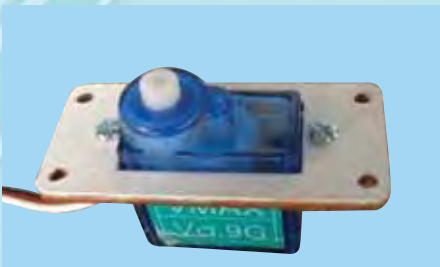
12B - Servo mounted to BACK SIDE of servo tray.
