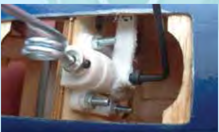
8E- Fasten the steering arm to the nose gear using an allen key to tighten the hex head set screw.
