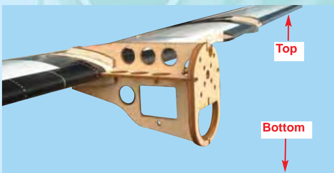
1G- Install the engine mount and hold in place while the epoxy cures.
