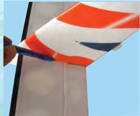
5D- Mark the outline of the vertical stabilizer onto the horizontal stabilizer.
