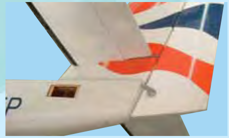
11G- Using 30 minute epoxy install the rudder control horn to its location in the rudder
