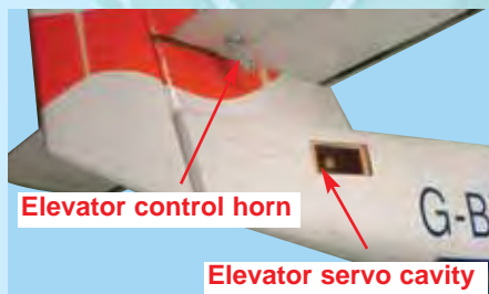
12D- Elevator servo location
