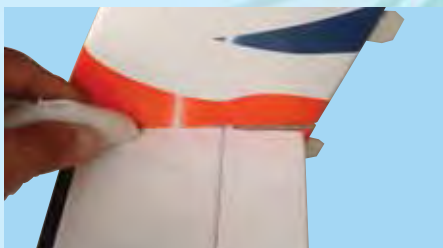
5K- Clean off any excess epoxy with a rag or tissue before it cures.
