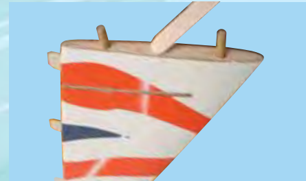
4C - Apply 30 minute epoxy to the bottom plate and dowels of the vertical stabilizer.
