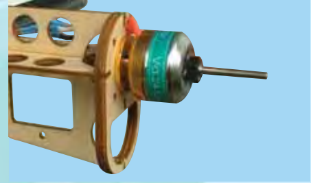
9C- Fasten the motor to the firewall using 4 bolts (3x10mm) & washer sets provided. Place washer on bolt and insert bolt through back of firewall & screw into tapped holes in motor mounting plate. Secure bolts with medium thread locker
