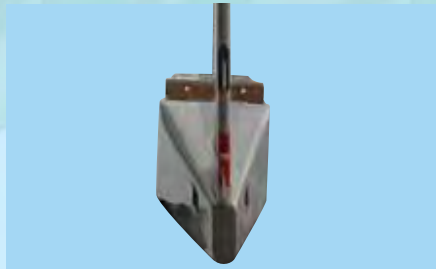
4D - Align the vertical stabilizer so that it is straight and at right angles to the top of the fuselage.
