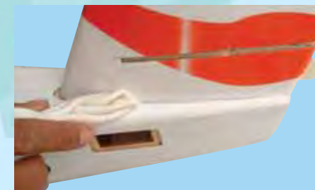
4E- Wipe off excess 30 minute epoxy
