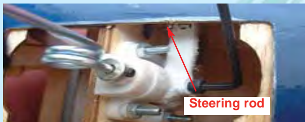
21.1 Nose steering arm connect to the steering rod
