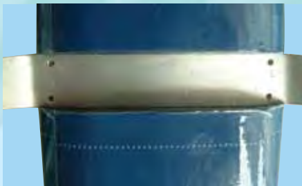
7C- Insert the pre-bent main landing gear into the fuselage
