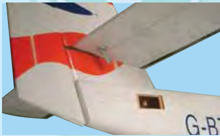
11E- Install the elevator control horn using 30 minute epoxy, washer and 2 x 10 mm screw.
