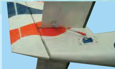
12E - Elevator servo attached to the fuselage and connected to the elevator control horn.
