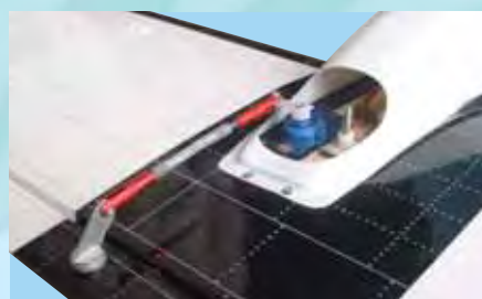
13E- Connect the aileron control rod between the servo arm and the control horn
