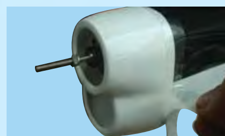
10F- Use transparent tape to secure the cowl to the motor covers.
