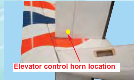
11D- Elevator control horn location
