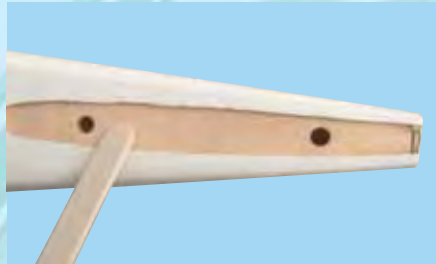
4B - Apply sufficient 30 minute epoxy into the slot in the fuselage.
