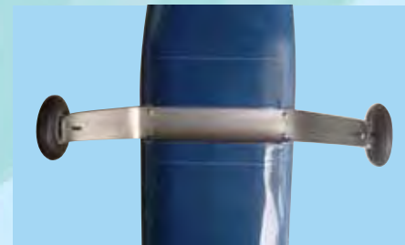
7D- Use four 10x2 mm screws to mount the main landing gear to the fuselage
