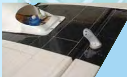
13D - Install the aileron control horn using 30 minute epoxy and the washer with 2 x 10 mm screw.
