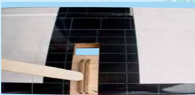
1E- Apply 30 minute epoxy to the top wing engine mount rail
