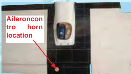
13B- Aileron control horn location
