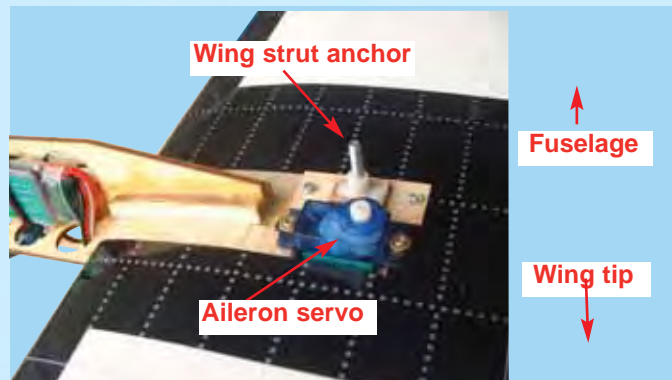
2B- Install servo using the rubber grommets & ferrules supplied with the servo.
