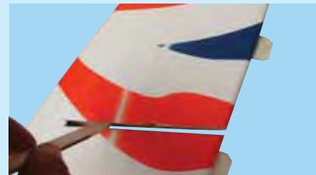
5I- Apply sufficient 30 minute epoxy into the slot of the vertical stabilizer.
