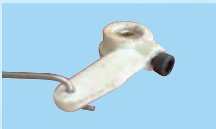
8B- Insert the steering rod Z-bend into the nose gear steering arm.
