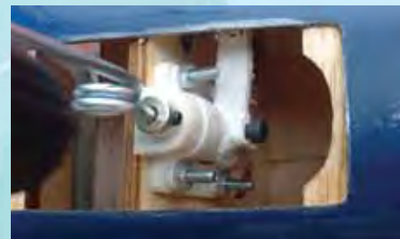
8D - Insert the nose gear through the nose gear bearing and steering arm.
