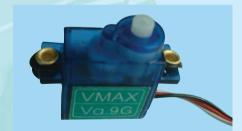
2A- Prepare the servos by fitting the rubber grommets & ferrules supplied with your servos
