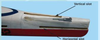
4A- The fuselage slots for the vertical & horizontal stabilizers
