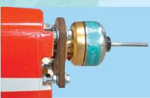
11J- Install four 3x30 [mm] bolt sets 11K- Thread four 3 mm nuts onto the 11L- Place four 3 mm washers on the bolts & then position the assembled power module. Secure in place with four more 3 mm washers & nuts. **Tighten snugly**
