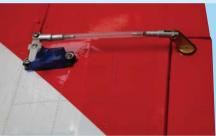
3C-Connect the aileron control rod between the servo arm and the control horn
