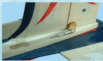
17A-Hold the rudder at neutral (not left, not right). Rotate the clevis to adjust the overall length. Then use the clevis screw to attach the clevis to the control horn. The clevis screw requires a 5/64 in. (2mm) hole. Secure the screw with thread lock
