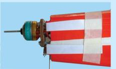
12A- Card stock strips overlying the 12B- Card stock strips overlying the cowl mounting tabs on the left side of the fuselage
