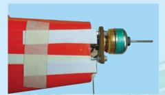
cowl mounting tabs on the right side of the fuselage
