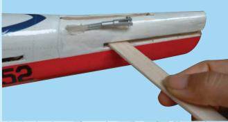
6H- Apply plenty of 30 minute epoxy into the horizontal
