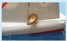
13E- Using 30 minute epoxy install the rudder control horn into the pre-cut slot
