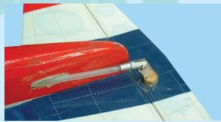
16B- Hold the elevator at neutral (not up, not down). Rotate the clevis to adjust the overall length. Then use the clevis screw to attach the clevis to the control horn. The clevis screw requires a 5/64 in. (2mm) hole. Secure the screw with thread lock
