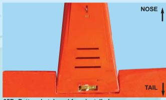
25D- Battery hatch and fuse installed
