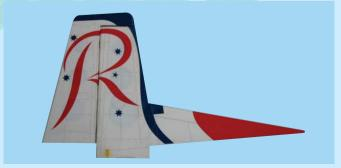
4C- Vertical stabilizer with pre-installed rudder
