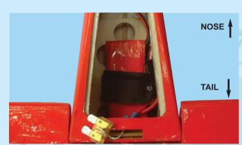
25C- Battery installed with fuse removed
