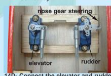
14D- Connect the elevator and rudder
