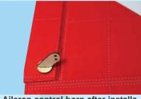
3B- Aileron control horn after installation.
