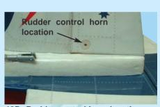
13D- Rudder control horn location
