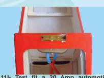
holder/switch to the fuselage by using spade fuse into the fuse holder/switch and then REMOVE THE FUSE
