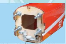
er-nut (front). Tighten the nuts securely & apply thread locker
