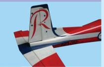
7A- Trial fit the vertical stabilizer into the fuselage slot
