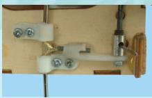
10C- Use four 2x10 [mm] screws to install the nose gear assembly. Then insert the control rod into the EZ connector and tighten the set screw
