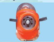
12D- Position the cowl over the mounting tabs. Note the strips are outboard. Align & center with respect to the motor shaft
