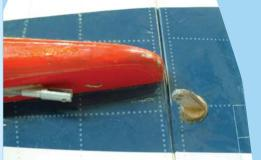
16A- Elevator control horn shown in position
