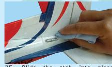
7F- Slide the stab into place & remove excess epoxy
