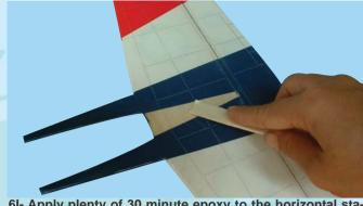
61- Apply plenty of 30 minute epoxy to the horizontal stabilizer
