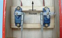
15A- Center the servo control surface and then connect the control rods to the servos using the clevises as
