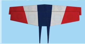
4B- Horizontal stabilizer with pre-installed elevator
