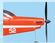
12G- With the BATTERY & FUSE **REMOVED** securely install the propeller
