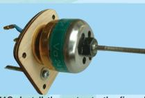
using 4 bolts (3x10mm) & washer sets provided. Place washer on bolt and insert bolt through back of firewall & screw into tapped holes in motor mounting plate. Secure bolts with medium thread locker
