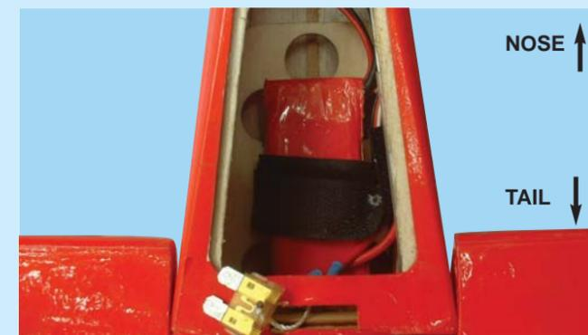
25C- Battery installed with fuse removed
