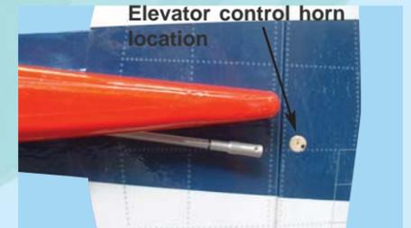
13B- Elevator control horn location
