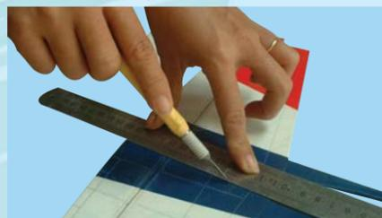
6D- Cutting inside the lines. **Do NOT cut the wood**
