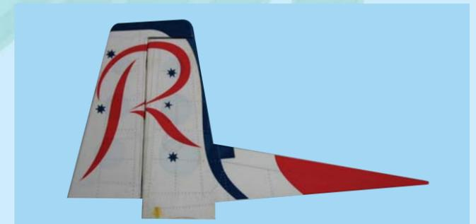
4C- Vertical stabilizer with pre-installed rudder
