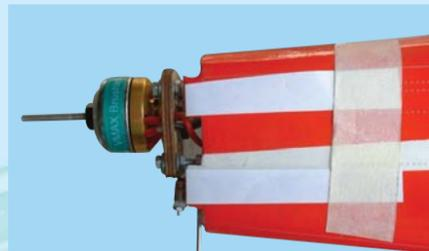
12B- Card stock strips overlying the cowl mounting tabs on the left side of the fuselage
