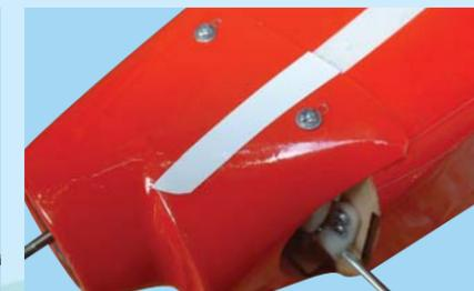
12F- Secure the cowl into place with four 2x10 [mm] screws
