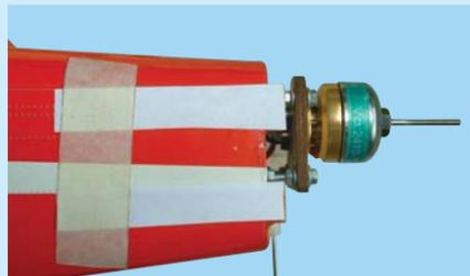
12A- Card stock strips overlying the cowl mounting tabs on the right side of the fuselage
