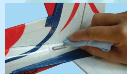
7F- Slide the stab into place & remove excess epoxy
