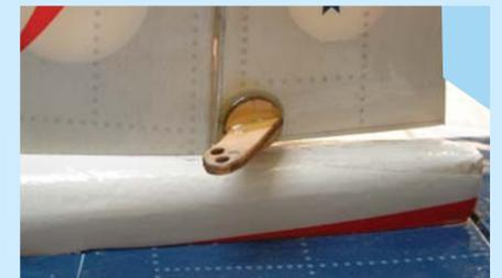
13E- Using 30 minute epoxy install the rudder control horn into the pre-cut slot
