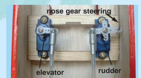
14D- Connect the elevator and rudder control rods to the servo arms
