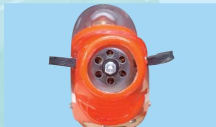
12D- Position the cowl over the mounting tabs. Note the strips are outboard. Align & center with respect to the motor shaft
