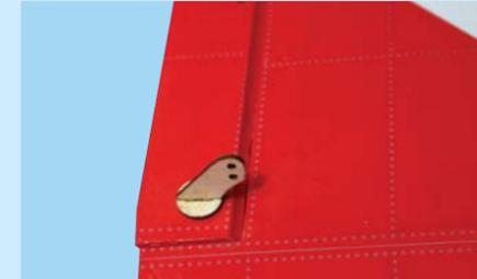
3B- Aileron control horn after installation.
