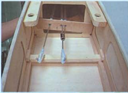
22.2 Pre-installed elevator and rudder pushrod
