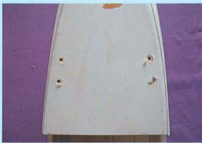
16.2 Turn over the fuselage to locate the 4 pre-drilled main landing gear mounting holes
