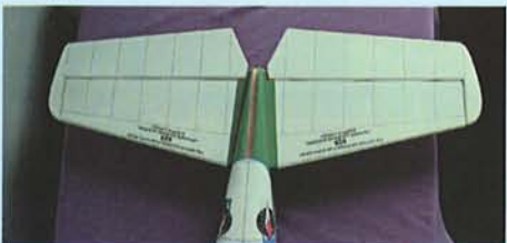
9.1 Trial fit the horizontal stabilizer in its slot
