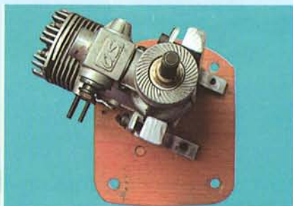
19.4 Engine and engine mount recommendation orientation.
