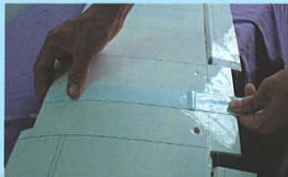
4.2 Carry on over the bottom of wing press down firmly as you go
