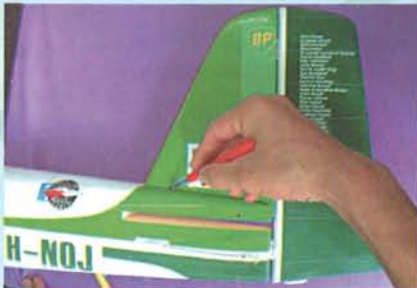
13.2 Mark both sides of the vertical stabilizer
