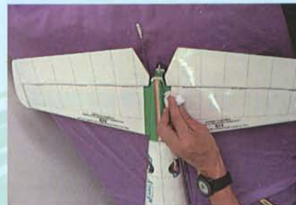
12.3 Wipe off excess epoxy
