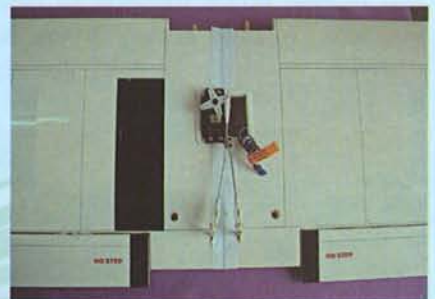
7.4 Final flap installation
