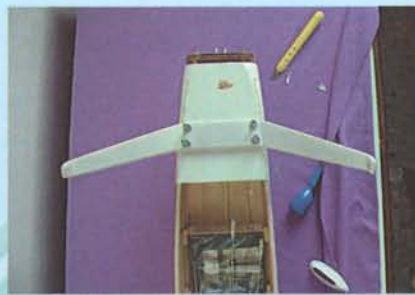
16.3 Use 4 metal sheet screws (5 x 35mm) to mount the main landing gear onto the fuselage
