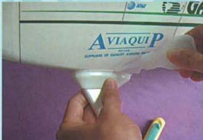
16.5 Use thick CA glue to glue the fairing to the fuselage
