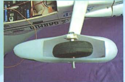
16.7 Install the wheel pan and wheel to the main landing gear
