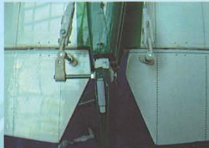
24.1 Rudder control horn installed and shown in position
