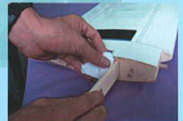
2.4 Wipe off the excess epoxy
