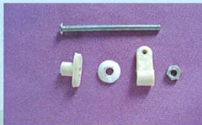
6.2 Aileron control horn assembly
