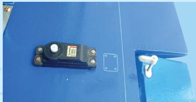
1C - Mount the aileron servos into the wing
