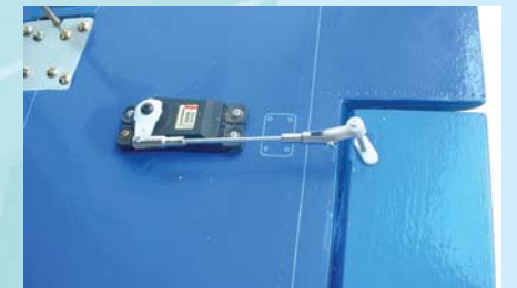
2C - Aileron control rod installed
