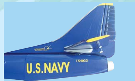
5E - Carefully press the vertical and horizontal stabilizer into the fuselage slot
