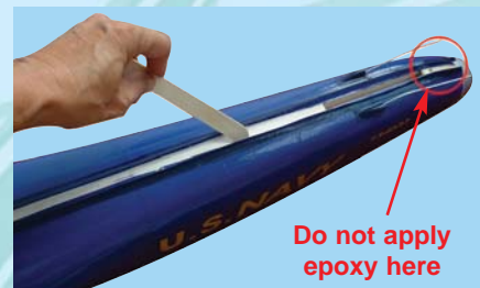
5B - Apply sufficient 30 minute epoxy to the exposed wood area in the fuselage
