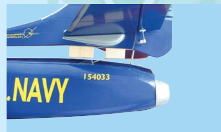
5D - Insert the vertical and horizontal stabilizer into the vertical slot
