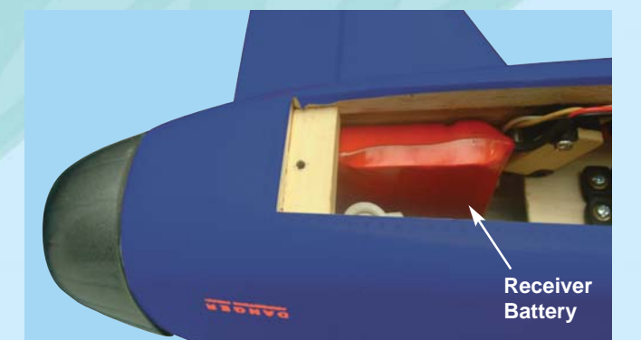
20B - Receiver battery and receiver location
