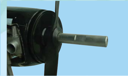
11C - Install the propeller, the prop washer and the prop nut
