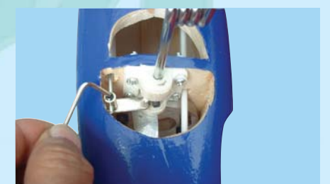
8D - Secure the EZ-connector to the nose gear push rod by tightening the set screw
