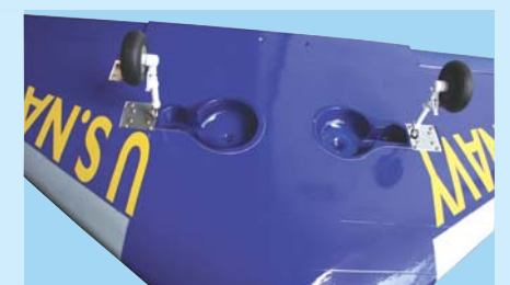
7D - Main landing gear mounted to both wings
