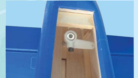
12D - Rudder control horn installed
