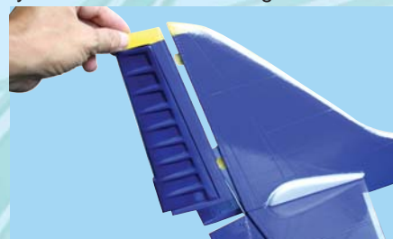
4E - Attach the rudder to the vertical stabilizer
