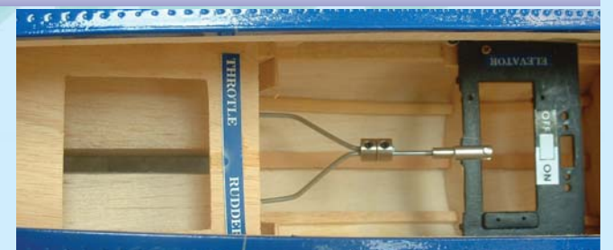
13A - Location of elevator, rudder and throttle servos
