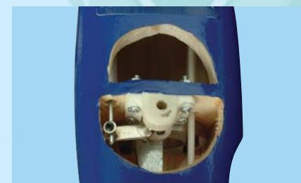
8B - Insert the nose gear push rod through the steering arm EZ-connector. Do not tighten yet
