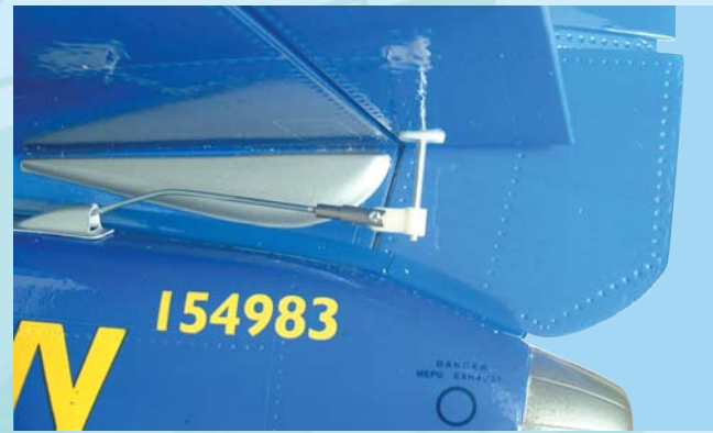
14B - Connecting the elevator control rods to the elevator
