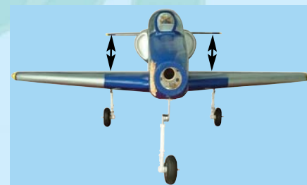
5F - Confirm that the horizontal stabilizer is level with respect to the wing
