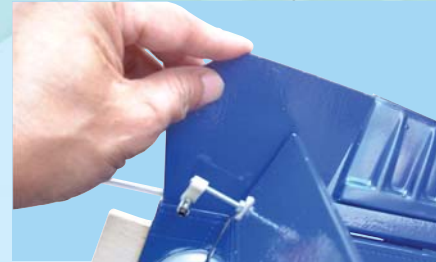
4H - Attach the lower rudder to the vertical stabilizer
