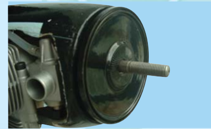
11B - Install the spinner backing plate
