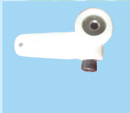
15A - Rudder control horn assembly
