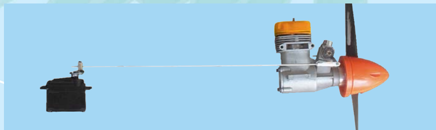
16B - The throttle servo controls the engine throttle using the throttle control rod
