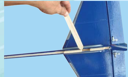
5C - Apply sufficient 30 minute epoxy to the exposed wood area in the vertical stabilizer
