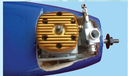
16A - Throttle control rod connected to the engine throttle arm
