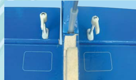
12C - Elevator control horns installed
