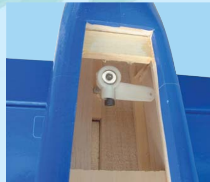
15B - Install the rudder control horn to the rudder control rod
