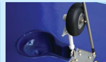
7C - Mounting the main landing gear to the wing
