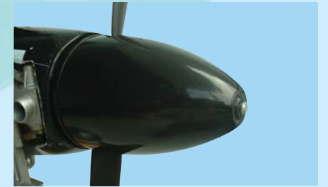
11D - Install the spinner cone using the retaining screw. Ensure the retaining screw is tight and secure
