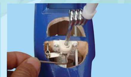
8C - Secure the steering arm to the nose gear wire by tightening the set screw
