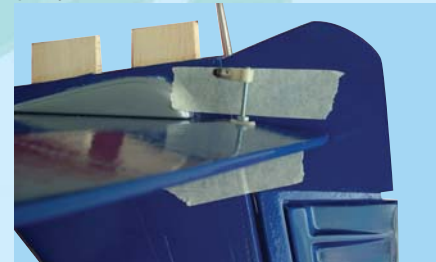
4I - Use the marking tape to align and hold the lower rudder in place
