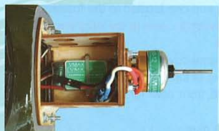
9M Mount the ESC to the fuselage
