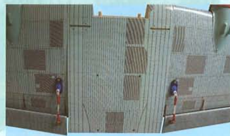
13C- Connect the flap control rod between the servo arm and the control horn
