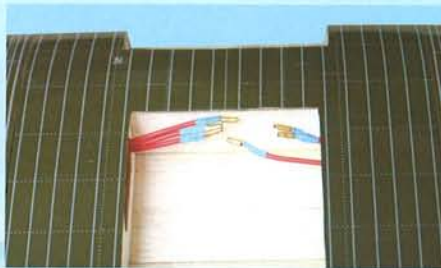
9H Both motor extension wire route through the pre-install tube guide to the wing center
