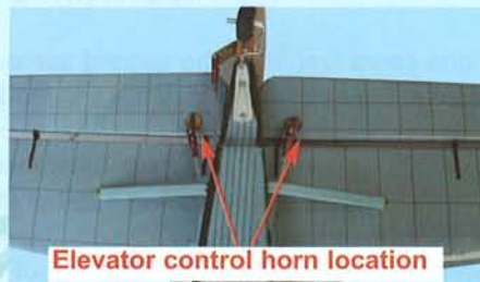
11D- Install the elevator control horn using 30 minute epoxy, washer and 2 x 12 mm screw.
