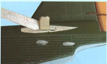
6F- Insert the horizontal stabilizer joiner then apply 30 minute epoxy to the expose wood area
