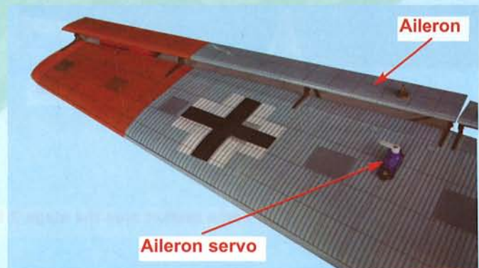
3B- Install servo using the rubber grommets & ferrules supplied with the servo.
