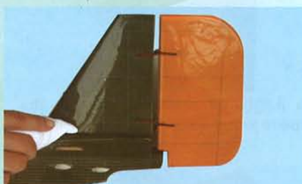
5E- Wipe off excess 30 minute epoxy
