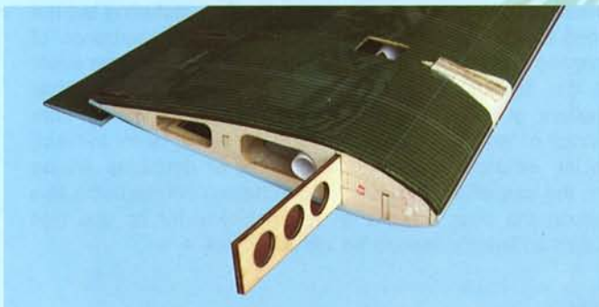
1E- Trial fit the wing joiner to the right wing panel
