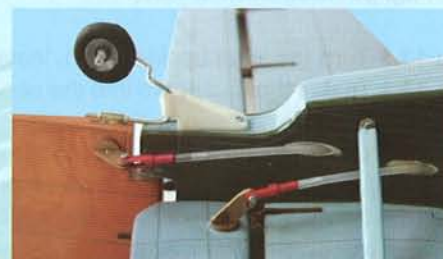
11E- Install the rudder control horn using 30 minute epoxy, washer and 2 x 15mm screw
