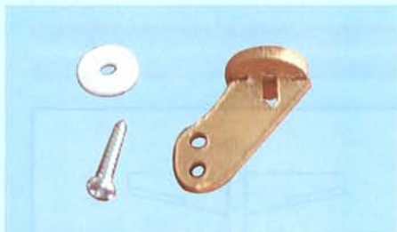
14A- Typical laser cut control horn assembly
