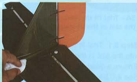
6I- Wipe off excess 30 minute epoxy
