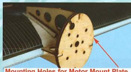
9B- A special pre-drilled firewall is included for mounting the recommended VMAX motor.
