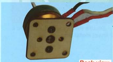
9D- using 2 short bolt (black) to the motor mounting plate
