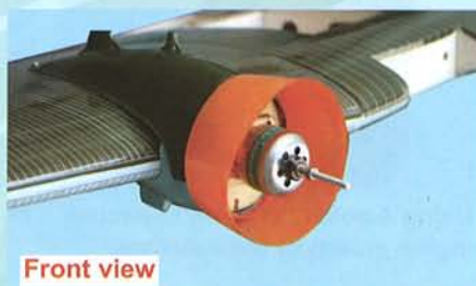
10D- Position the rear cowl over the engine covers. Align cowl & center about the motor shaft.
