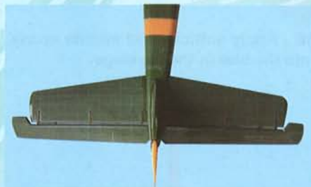
6H- Carefull insert both left and right horizontal stabilizer to the joiner ,make sure it align and square
