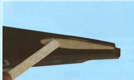
5B - Apply sufficient 30 minute epoxy into the slot in the fuselage.
