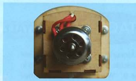
9J- Using 4 bolts (3x15mm) to secure the engine mounting plate to the engine mount
