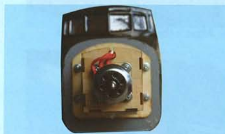
9K Using 4 bolts (3x15mm) to secure the engine mount to the fuselage
