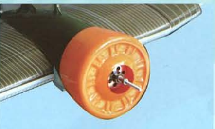
10E- Position the front cowl over the rear cowl. Align cowl & center about the motor shaft.
