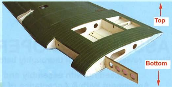
1D- Trial fit the wing joiner to the wing center panel
