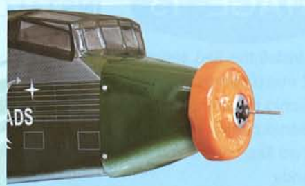
10C- Using four 2 x 10mm screws to secure the motor cover to the fuselage
