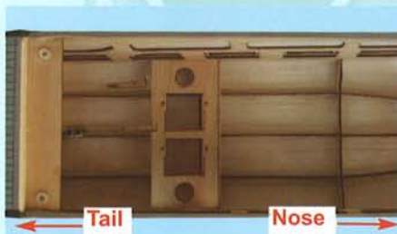
12A - Servo tray. 1 for Rudder servo. 1 for Elevator servo.
