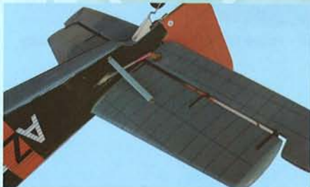
6J Turn over the fuselage then attache the horizontal struts to the horizontal stabilizer
