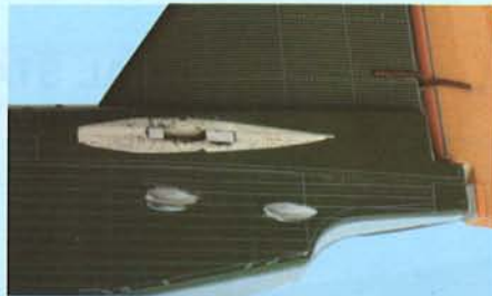
6E- Carefull cut through the covering (Do NOT cut the wood), then remove the covering
