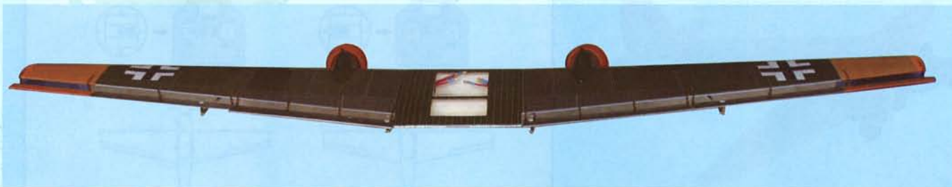
13F - Wing with aileron and flap in neutral position
