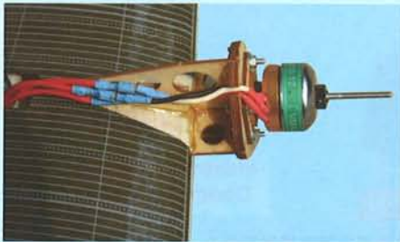
9G Connect the motor extension wire on both left and right motor
