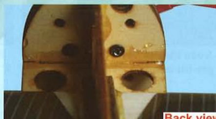
9E- Using 2 long bolt (black) to mount the motor mounting to the engine mount
