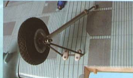
7C- Insert the pre-bent main landing gear into the slot then secure with 2 straps and 4 screws
