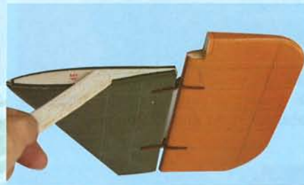
5C - Apply 30 minute epoxy to the bottom plate and dowels of the vertical stabilizer.
