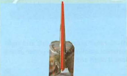
5D - Align the vertical stabilizer so that it is straight and at right angles to the top of the fuselage.
