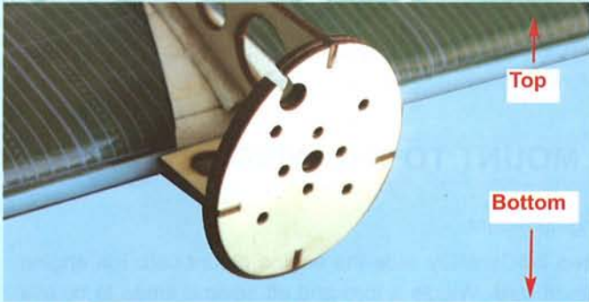
2G- Install the engine mount and hold in place while the epoxy cures.
