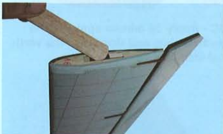
6G Apply 30 minute epoxy to the expose wood area
