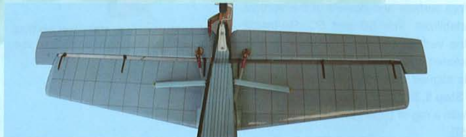
6K attache the struts to the both horizontal stabilizer
