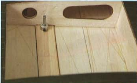
7D- Install the strut and secure with the collar
