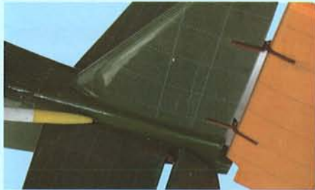
6D- Mark the outline of the horizontal stabilizer right and left panels
