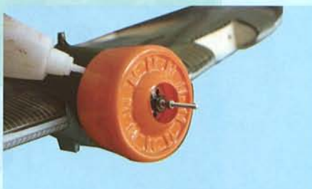
10F- Use CA glue to secure the cowl to the motor covers.
