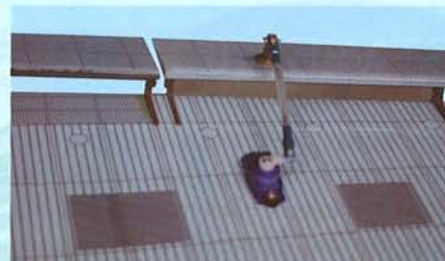
13C- Connect the aileron control rod between the servo arm and the control horn
