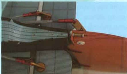
12D- Elevator & rudder clevises connect to the elevator and rudder control surface
