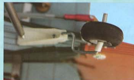
8D - Secure the tail wheel with two 2 x 10 sheet metal screws
