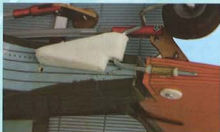
8C- Slide the tail wheel assembly into the pre-installed sleeve tube
