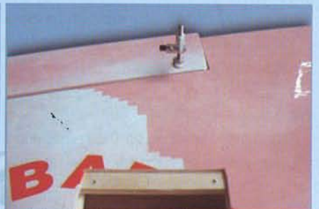
2.E Install aileron control horn
