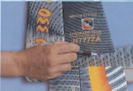
10.A Mark both sides of the vertical stabilizer
