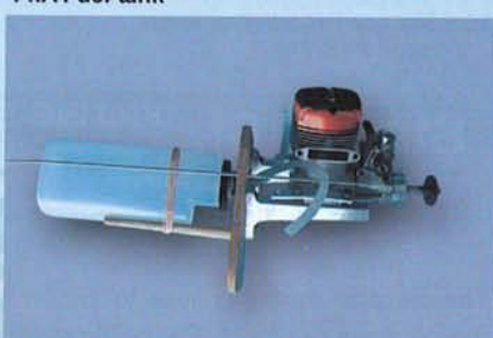
14.D Fuel tank installed on the power module
