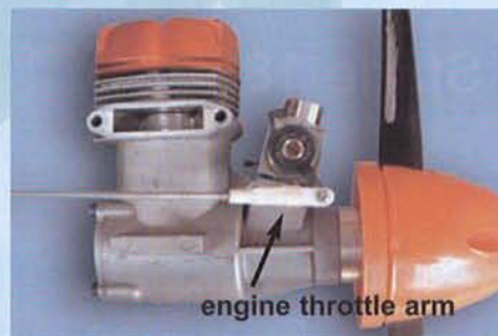
21.B Throttle control rod connected to the engine throttle arm
