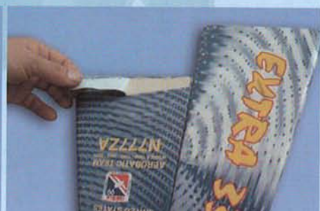
10.C Remove covering from both sides
