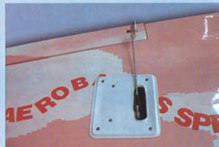
3.C Aileron control installed
