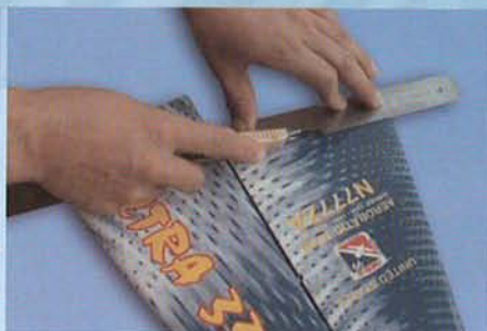
10.B Carefully cut through the covering
