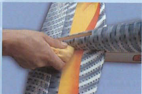
8.C Wipe off excess epoxy
