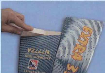
11.A Apply plenty of epoxy
