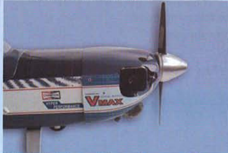
15.I Install the muffer and connect the fuel and pressure line
