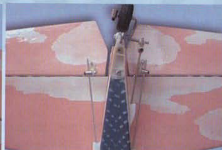
19.B Connecting the elevator pushrods to the control horns
