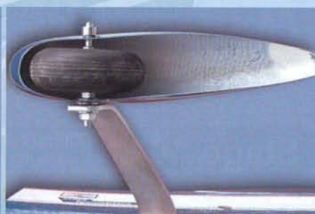
12.D Install the wheel pant and wheel to the main landing gear
