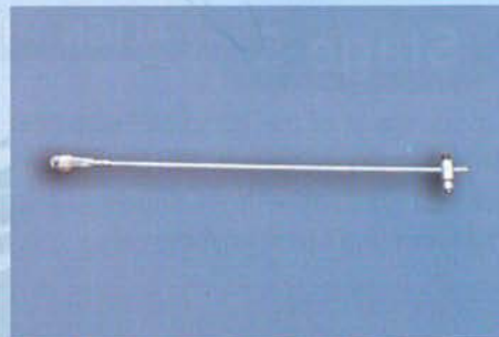
3.A Aileron control rod assembly
