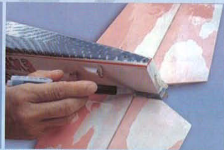
6.B Mark the bottom of the horizontal stabilizer
