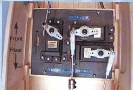
18.A Position of throttle, rudder and elevator servos and connected to the pushrods.
