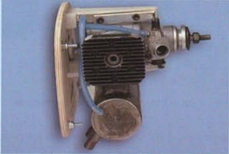
15.E Engine and engine mount recommendation orientation.
