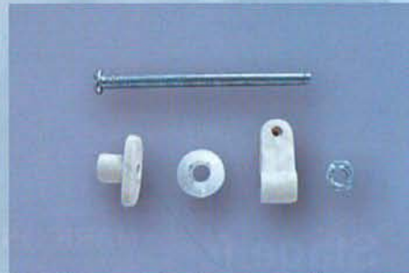
3.B Aileron control horn assembly
