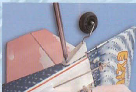
13.B Screw the tail wheel assembly to the fuselage
