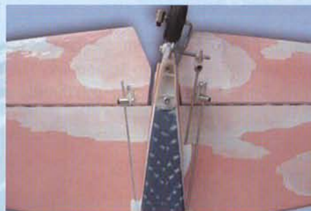
20.B Connecting the rudder pushrod to the rudder control horn
