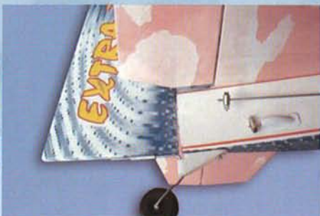
16.C Rudder control horn location
