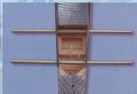
1.D Insert the wing spar joiner tubes into the fuselage.
