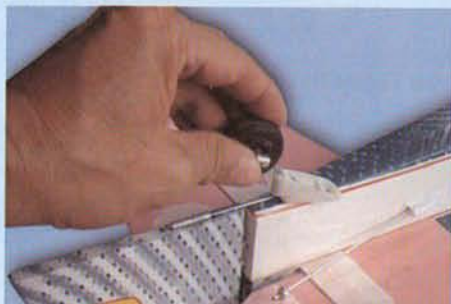
13.A Insert the tail wheel steering wire into the steering guide tube
