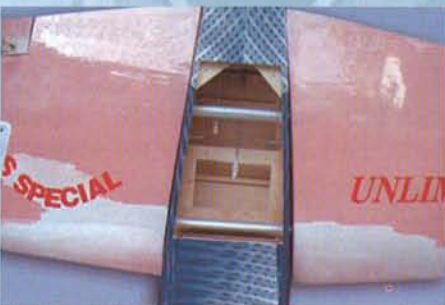
1.F Plug-in both wing panels
