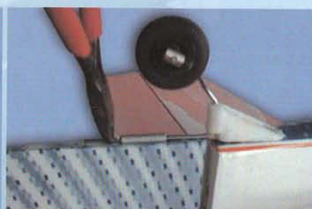
13.C Trim off the excess tail steering wire
