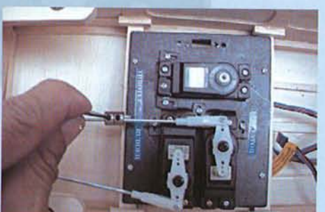
19.C Loosen collars to align elevator surfaces. Tighten collars securely
