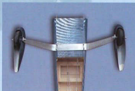
12.E Use 4 metal sheet screws (5 x 35mm) to mount the main landing gear onto the fuselage
