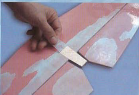
7.D Remove covering from the bottom surface
