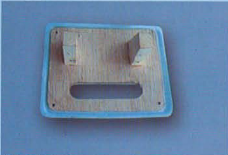
2.C Aileron servo mount
