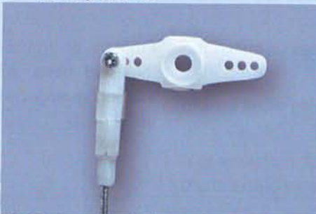
18.C Connecting clevis to the servo arm
