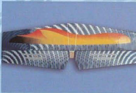
7.A Lines marked on the horizontal stabilizer
