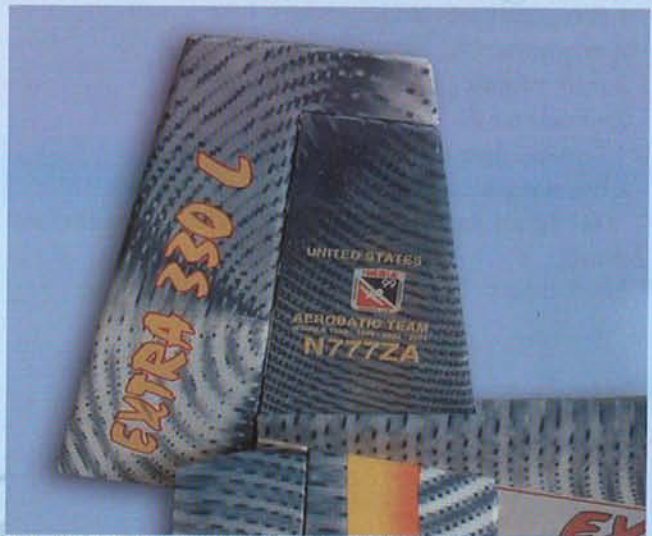
9.A Trial fit the vertical stabilizer onto fuselage.
