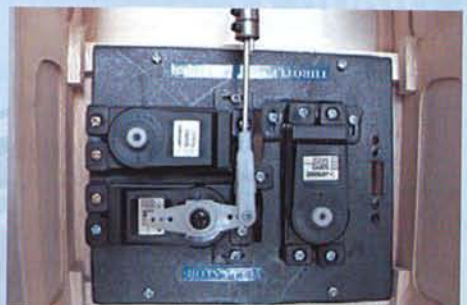
18.D Connecting the elevator pushrod to the elevator servo arm
