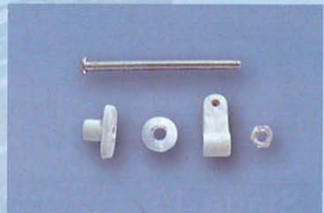
16.A Control horn assembly
