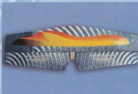
4.B Horizontal stabilizers with pre-installed elevator
