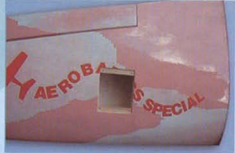
2.B Aileron servo location
