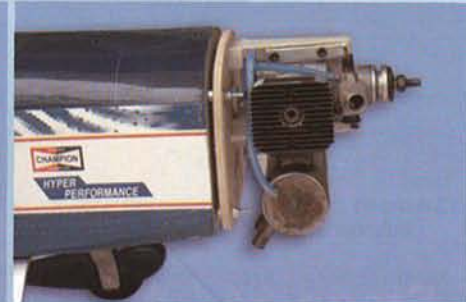
15.G Throttle control connect to the engine
