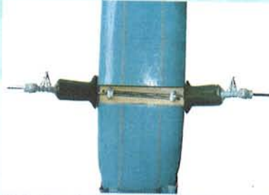
13.3 Use 4 sheet metal screws and 2 traps to mount the main landing gear onto the fuselage
