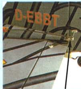
17.3 Rudder control horns location
