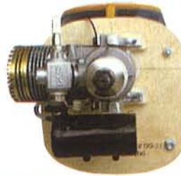
16.8 Install the muffer and connect the fuel and pressure line
