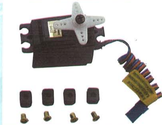
2.1 Prepare the servos by fitting the rubber grommets & ferrules supplied with your radio
