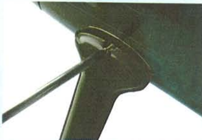
13.5 Mount the main landing gear fairing with 2x10 screw
