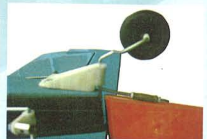
14.3 Trim off the excess tail steering wire
