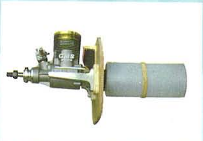
16.5 Engine and fuel tank positioned on the power module
