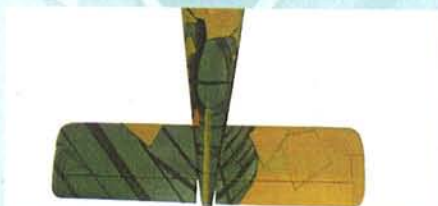
6.1 Trial fit the horizontal stabilizer in its slot
