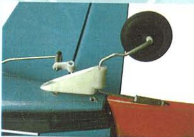
14.1 Insert the tail wheel steering wire into the steering guide tube
