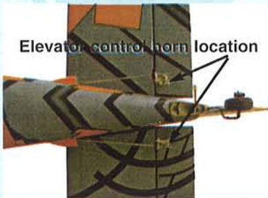
17.2 Elevator control horn location
