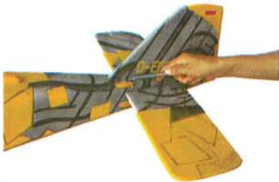
11.1 Mark both sides of the vertical stabilizer
