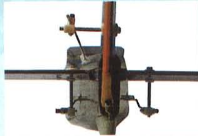
20.1 Two independent elevator control horns shown in position
