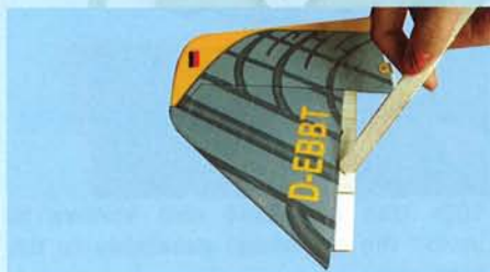
7E- Apply plenty of 30 minute epoxy
