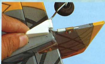
10C- Insert the tail wheel to the sleeve tube
