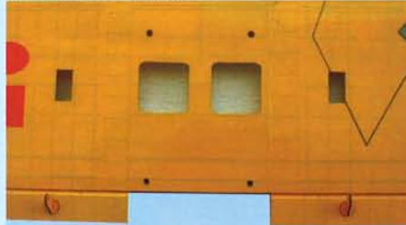
3B- Aileron control horn after installation.
