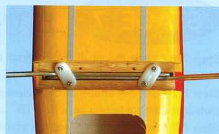
9D- Use two straps and four 10x2 [mm] screws to mount main landing gear assembly to the fuselage
