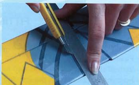
6D- Cutting inside the lines. Do NOT cut the wood
