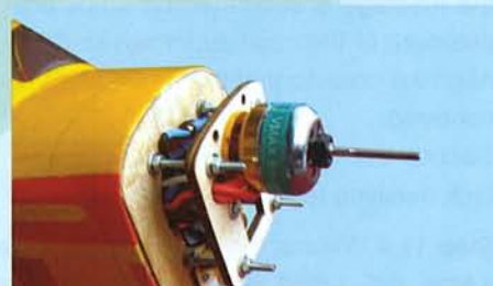
11L- Place four 3 mm washers on the bolts & then position the assembled power module. Secure in place with four more 3 mm washers & nuts. Tighten snugly
