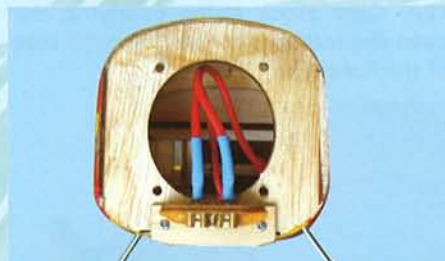
11H- Mount the pre-assembled fuse holder/switch to the fuselage by using two 2x8 [mm] screws
