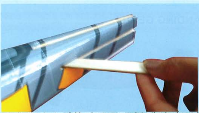
6H- Apply plenty of 30 minute epoxy into the horizontal slot
