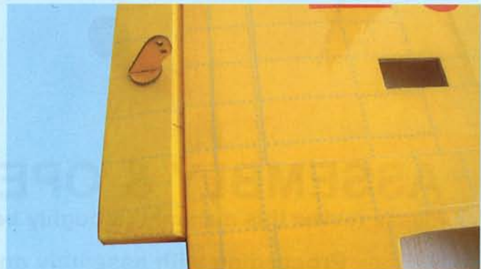
1D- Control horn installation to the aileron
