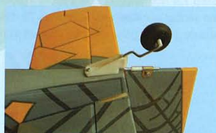
10D- Use two 2x10 mm screws to install the tail wheel assembly to the fuselage
