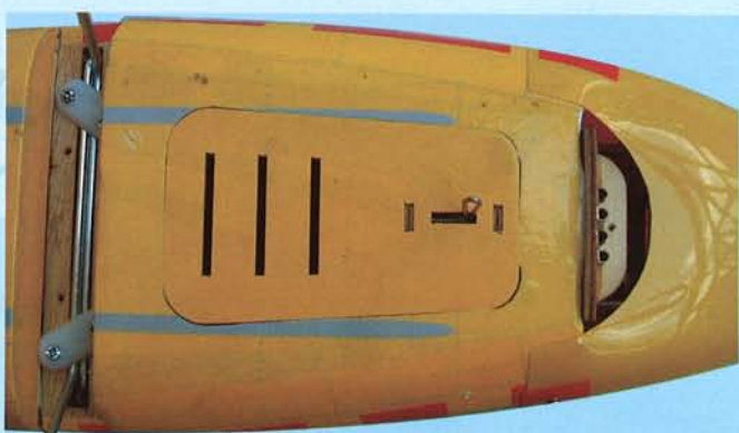
25D- Battery hatch installed
