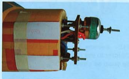
12A- Card stock strips overlying the cowl mounting tabs on the right side of the fuselage
