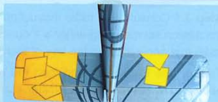
5A- Trial fit the horizontal stabilizer in its slot
