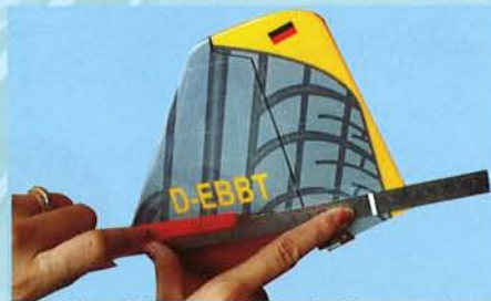
7C- Carefully cut through the covering. Do NOT cut the wood
