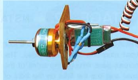
11F- Completed power module assembly with motor and electronic speed control installed
