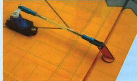
3C-Connect the aileron control rod between the servo arm and the control horn
