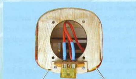
11I- Test fit a 20 Amp automotive spade fuse into the fuse holder/switch and then REMOVE THE FUSE
