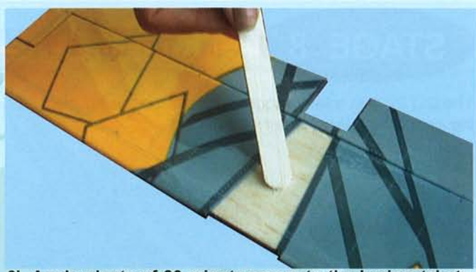
6I- Apply plenty of 30 minute epoxy to the horizontal stabilizer
