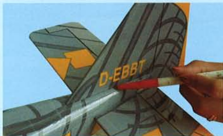
7B- Mark both sides of the vertical stabilizer
