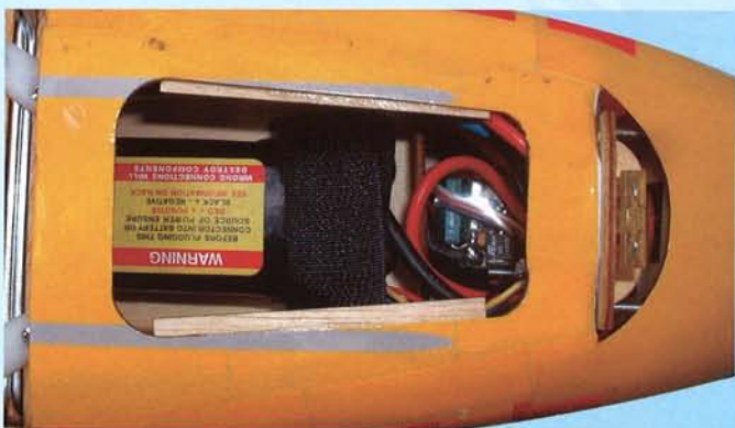
25C- Battery installed
