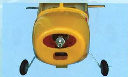
12D- Position the cowl over the mounting tabs. Note the strips are outboard. Align & center with respect to the motor shaft
