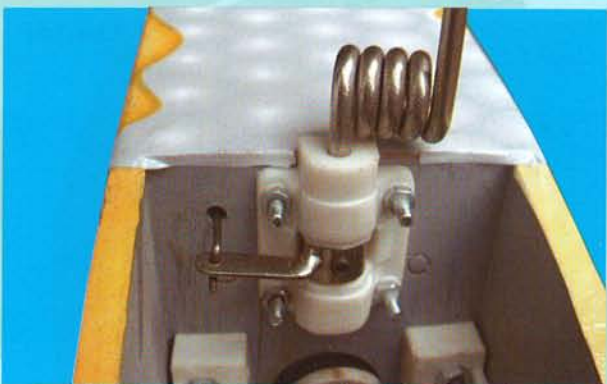
15F- Typical nose gear installation when complete.
