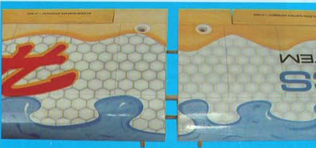
2B- Align the two wing panels and slowly close the gap until the wing root ends are firmly in contact with each other
