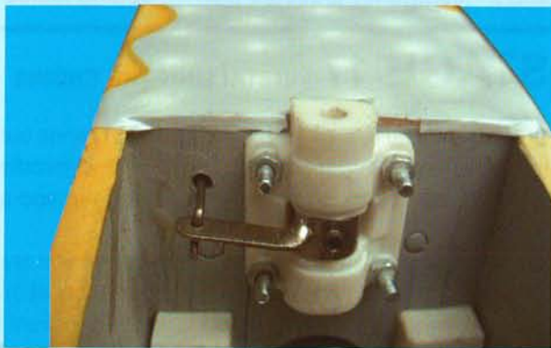
15D- Place the steering arm into the slot in the nylon nose gear bearing
