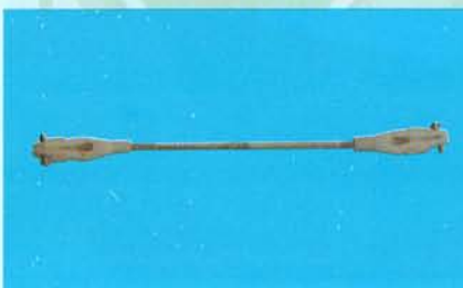
5A- Aileron control rod assembly
