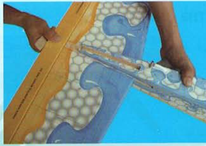
10C- Slide the horizontal stabilizer in place
