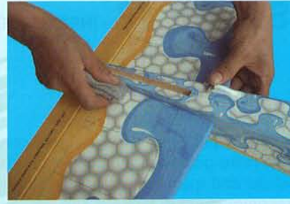
10D- Wipe off excess epoxy
