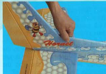
12B- Slide the stab into place & remove excess epoxy
