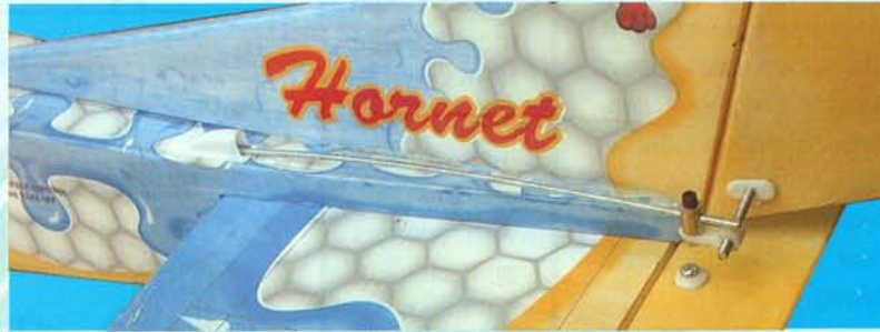
25A - The rudder pushrod is connected to the rudder control horn
