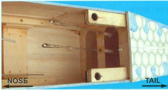
23B- Pre-installed elevator, throttle and rudder pushrod
