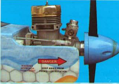
18A- Clevis attached to engine throttle arm
