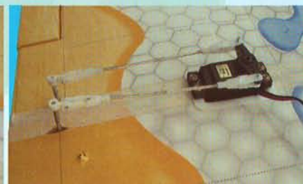
5C- Aileron servo and control rods installed.
