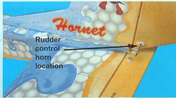
21D- Rudder control horn location
