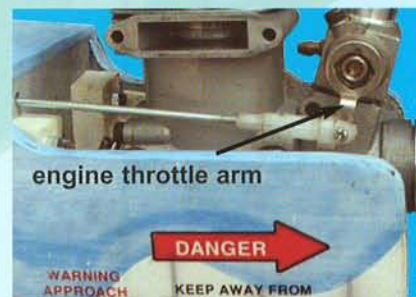
26B- Throttle control rod connected to the engine throttle arm
