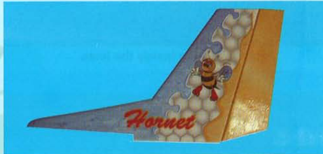
6C- Vertical stabilizer with pre-installed rudder
