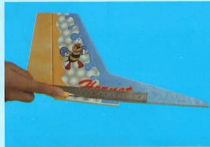
11C- Carefully cut through the covering
