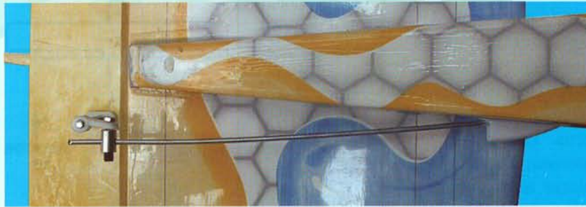
24B- Loosen the set screw to connect the elevator pushrod to the elevator control horn, align the elevator surface so that it is level with the plane of the horizontal stabilizer, then tighten set screw securely.
