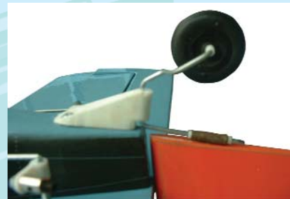
17.3 Trim off the excess tail steering wire
