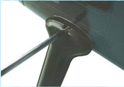
16.5 Mount the main landing gear fairing with a 2x10 screw
