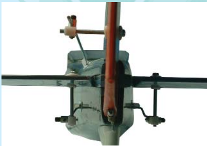
23.1 Two independent elevator control horns shown in position
