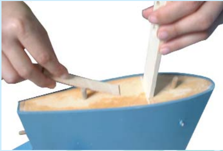
3.1 Apply plenty of glue 30 minute epoxy to joiner & both wing roots.
