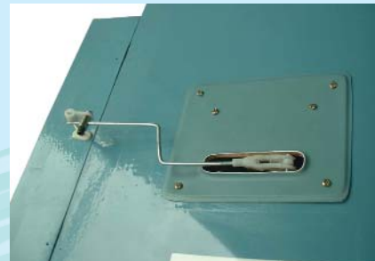
7.4 Final flap installation
