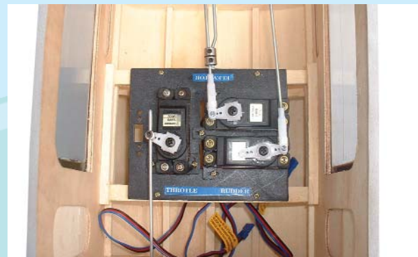
21.3 Throttle, elevator and rudder servos connected to their respective push rods
