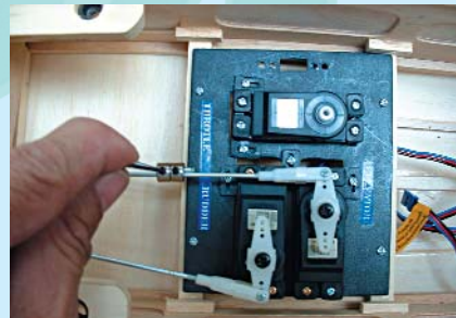
23.3 Loosen collars to align elevator surfaces. Retighten collars securely
