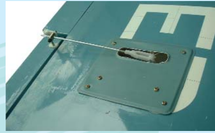
6.3 Aileron control rod installed
