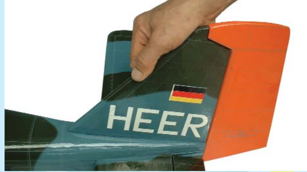
15.2 Slide the vertical stabilizer into place
