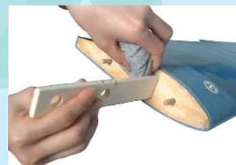
2.4 Wipe off any excess epoxy that squeezes out.
