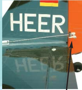
20.3 Rudder control horn location
