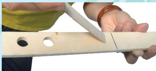
2.1 Apply epoxy to one end of wing joiner
