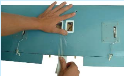
4.1 Apply tape over the joint, starting here.
