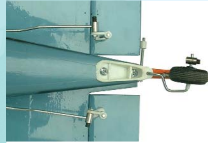
20.4 Elevator and rudder control horn connected to the control rod
