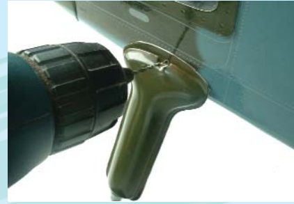
16.4 Drill pilot holes with a 1/16 (or 1,6 mm) drill-bit
