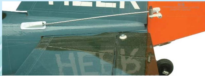
24.2 Connecting the rudder pushrod to the rudder control horn
