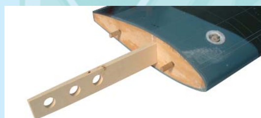
2.2 Carefully insert the joiner... Also the dowel guides...
