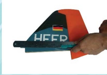
14.2 Carefully cut through the covering. Do NOT cut the wood.
