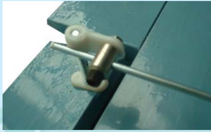
6.2 Aileron control horn assembly
