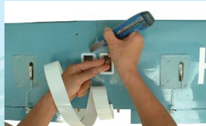
4.3 Trim off any excess trim tape.
