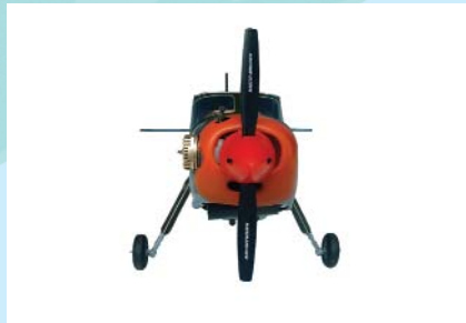
19.8 Install a suitable prop and spinner
