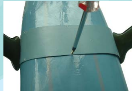
16.7 Install the main landing gear cover using 6 screws.
