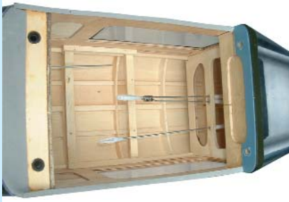
22.2 Pre-installed elevator and rudder pushrod
