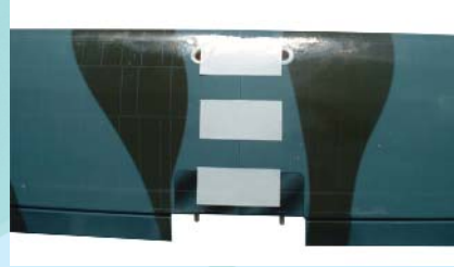
3.4 Use tape to hold tightly together
