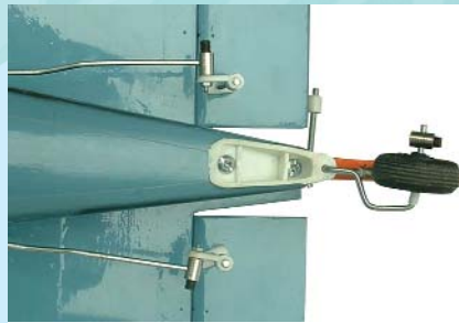
23.2 Connect the elevator pushrods to the control horns
