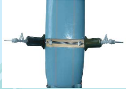
16.3 Use 4 sheet metal screws and 2 straps to mount the main landing gear onto the fuselage
