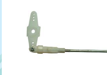
22.3 Connect a clevis to the servo arm
