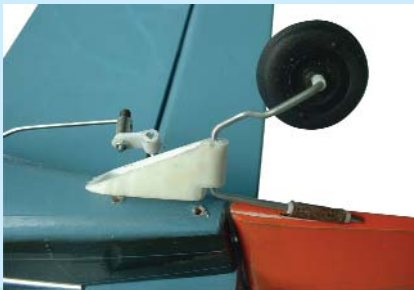
17.1 Insert the tail wheel steering wire into the steering guide tube
