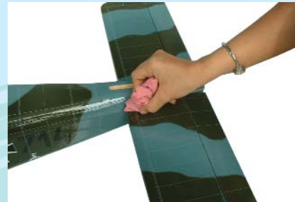
12.3 Wipe off excess epoxy
