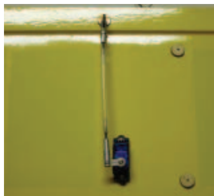
Separate aileron servos provide precise control because of the short, straight linkage.
