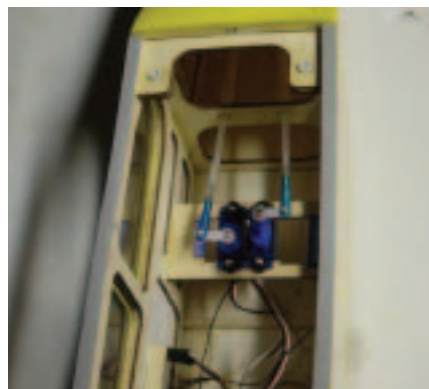
The rudder and elevator servos are mounted on a lite-ply tray. Note the precision-laser-cut wood construction.
