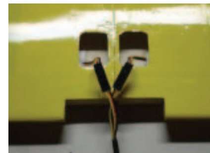
The Cub is equipped with dual aileron servos, and I used a Y-harness to connect the servos to the receiver instead of mixing them.
