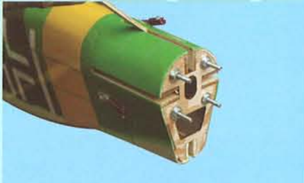
8D- Apply sufficient 30 minute epoxy to the exposed wood in the top vertical slot
