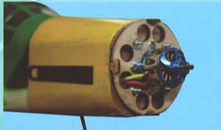
11G- The front motor mount with the motor install to the nose
