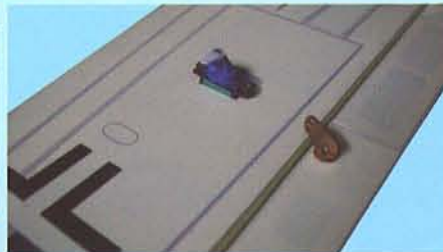
21B- Install the flap servos and flap control horns
