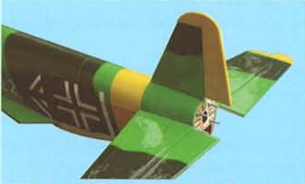
8A- Trial fit the top vertical stabilizer into the slot in the top of the fuselage.
