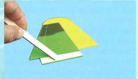
8C- Apply sufficient 30 minute epoxy to the exposed wood in the top vertical exposed wood area
