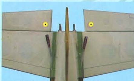
12A- Elevator control horn location
