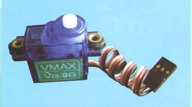
4A- Prepare the servo by fitting the rubber grommets & ferrules supplied with your radio
