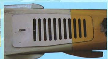
22A- Battery hatch installed
