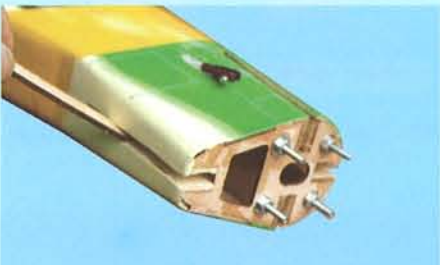
8H- Apply sufficient 30 minute epoxy to the exposed wood in the bottom vertical slot
