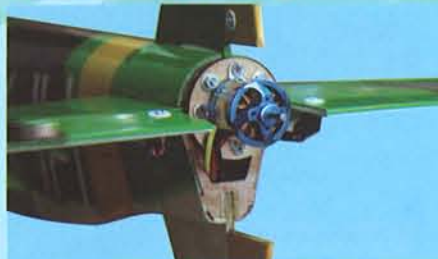
11G- The rear motor mount with the motor install to the rear end
