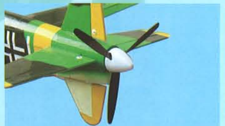
11H- Cowl, propeller and spinner installed to the rear end
