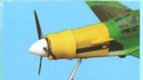
11H- Cowl, propeller and spinner are installed to the nose
