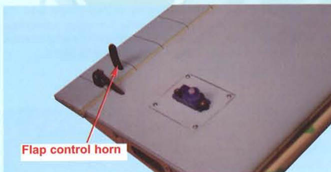
1G - Install flap servo mount to the wing panel
