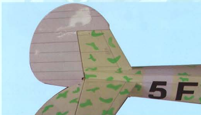
6A- Trial fit the vertical stabilizer in its slot
