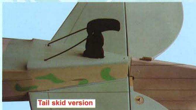
7C- Use 30 minute epoxy to install the tail skid to the fuselage
