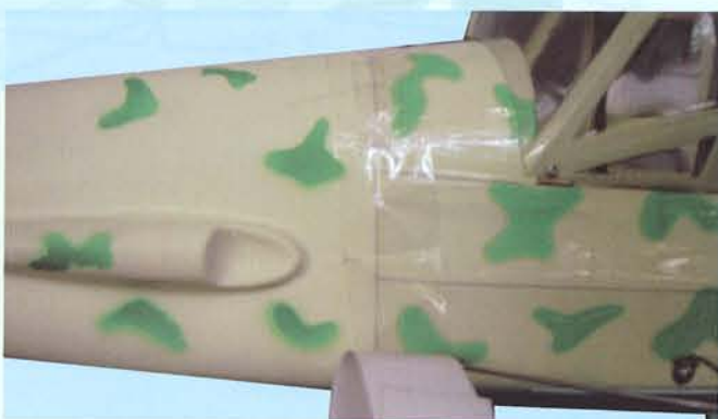
16D- Use transparent tape to secure the cowl to the fuselage
