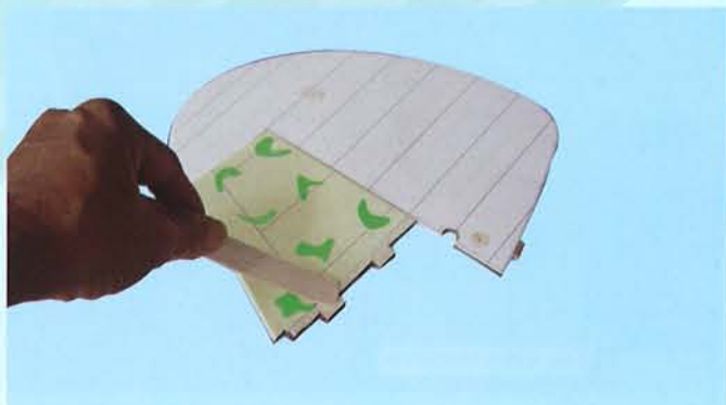
6F- Apply plenty epoxy to the exposed wood on both sides of the vertical stabilizer
