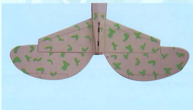
5C- Trial fit the horizontal stabilizer to the fuselage
