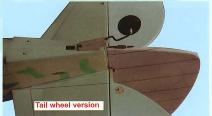
7D- Use two 2 x 8 screws to mount the tail wheel to the fuselage
