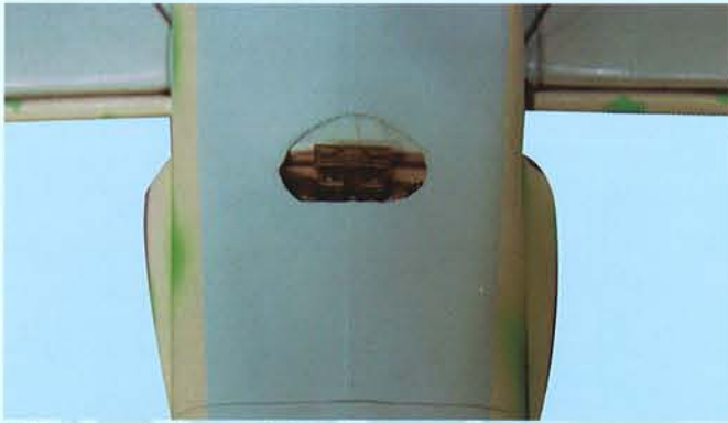
11C- Install the cowl already cut for the fuse exit
