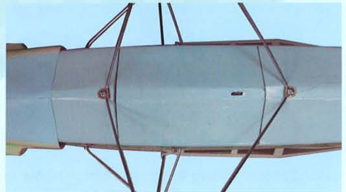
10D- Battery hatch installed
