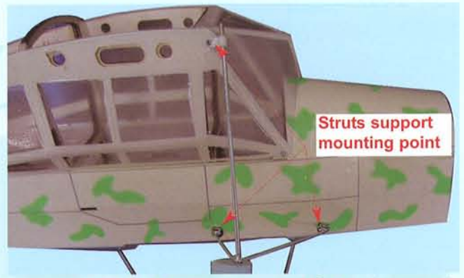
2E- Use three 2 x 8 screws to mount the struts support to the fuselage
