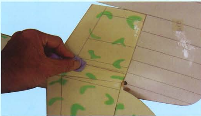
6G- Slide the vertical stabilizer into place. Wipe off any excess epoxy
