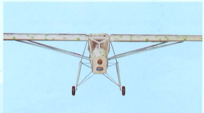
3J - Right and left wing struts mount to the wing and fuselage
