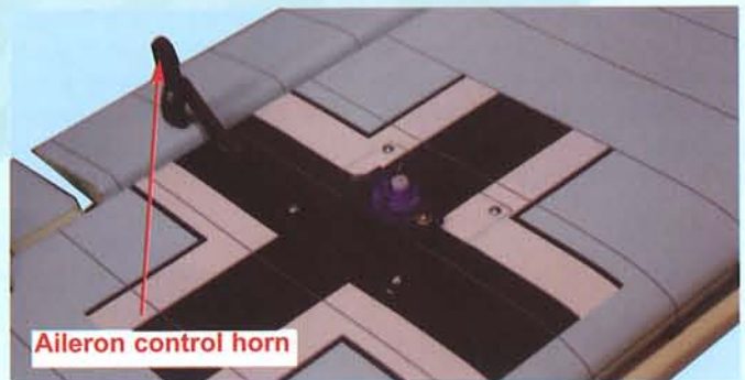
1H - Install aileron servo mount to the wing panel
