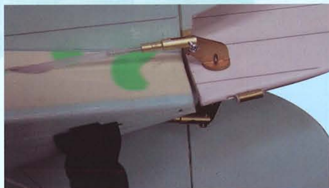
11D - Rudder control horn and control rod installed
