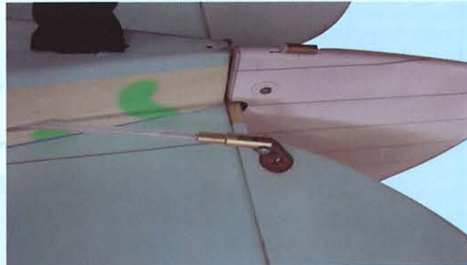
11F - Elevator control horn and control rod installed
