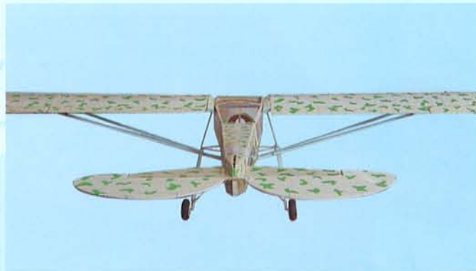
5K- Make sure the horizontal stablizer sqare and level
