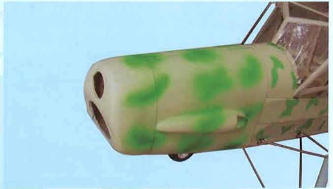
11D- Cowl install to the fuselage
