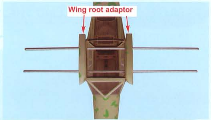
3F- Insert the wing root adaptor to the wing joiner
