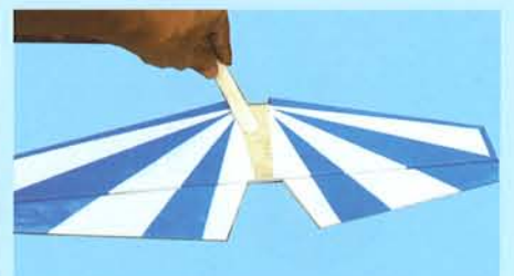
7C- Apply sufficient 30 minute epoxy to the exposed wood on both side of the horizontal stabilizers.
