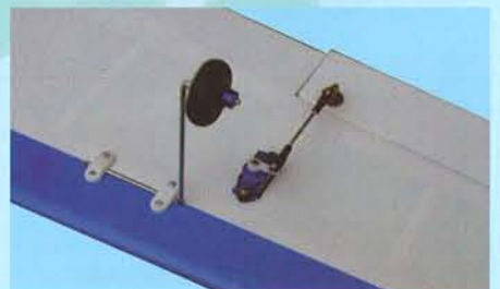
10C- same as the left wing mount the wing console gear to the right wing
