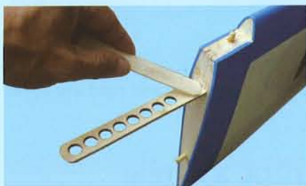
2A- Apply plenty of 30 minute epoxy to all surfaces
