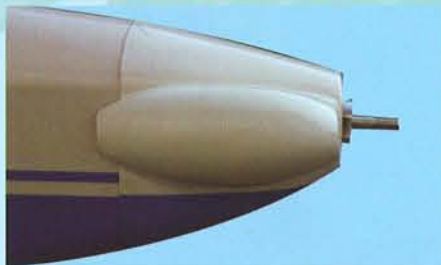
12H- Use transparent tape to secure the cowl to the fuselage
