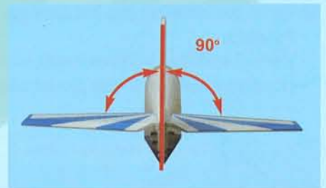
8F- Before the epoxy cures, confirm the both vertical stabilizer is at 90 degrees with respect to the horizontal stabilizer
