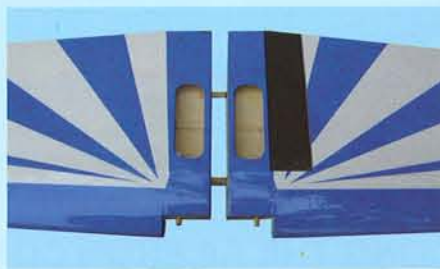
2B - Align the wing panels and slowly close the gap until the wing roots are firmly in contact with each other.
