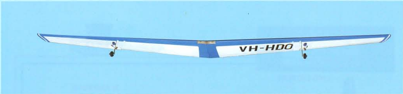
10D- Wing console gear mount to the wing
