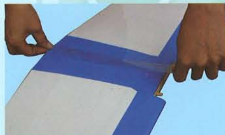
3A - Straddle the wing joint tape over the wing joint starting here on the bottom of the wing.
