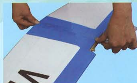
3B - Continue around the wing. Ensure the tape straddles the joint.
