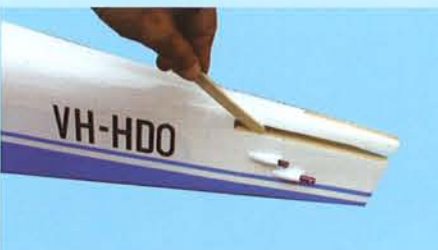
7D- Apply sufficient 30 minute epoxy to the exposed wood on the horizontal slots
