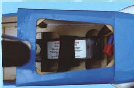
22A- Battery in its locations
