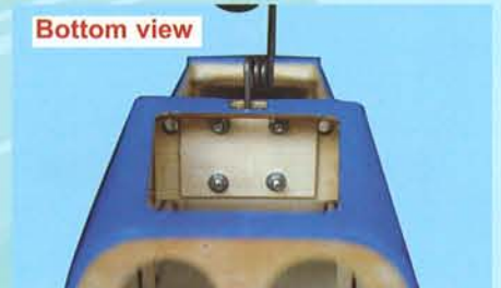
9C- Using 4 (3 x 15 mm) to mount main landing gear to the fuselage
