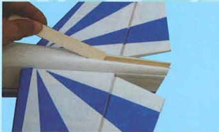
8D- Apply sufficient 30 minute epoxy to the vertical slot
