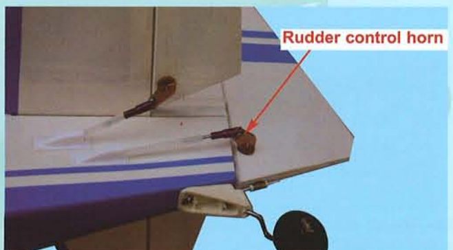
13D- Connect rudder control rod to the rudder control horn
