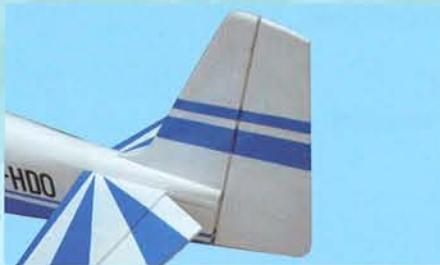
8E- Insert the top vertical stabilizer to the top vertical slot, clean of the excess epoxy
