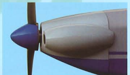
12I- Install the propeller and spinner
