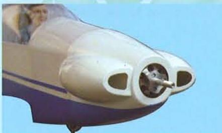
12G- Mount the cowl to the fuselage
