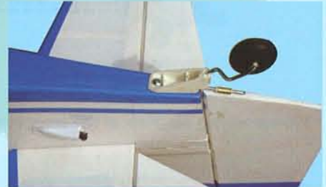
11C- Tail wheel mount to the fuselage
