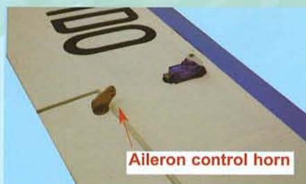
5B- Aileron control horn and servo
