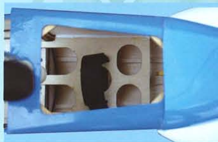
22A- Battery locations
