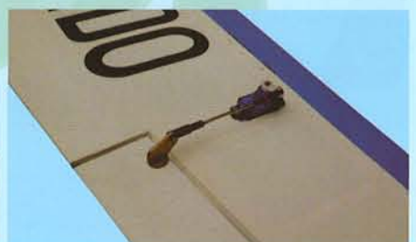
5C- Aileron control rod installed
