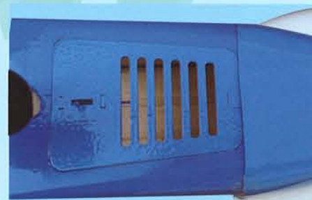
22A- Battery hatch installed
