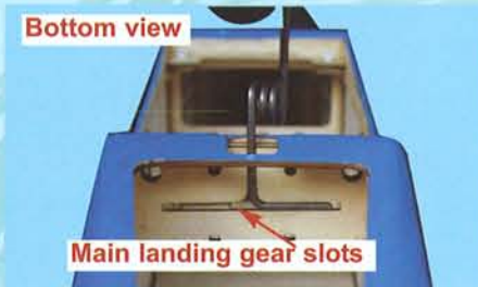
9B- Fit main landing gear into its location
