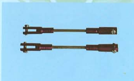
5A- Aileron control rod assembly
