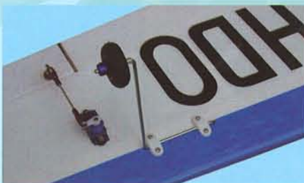
10B- Using 2 plastic strap and 4 metal screws 2 x 10mm to mount the wing console gear to the left wing
