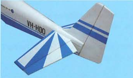
8A- Trial fit vertical stabilizer into the slot in the of the fuselage.
