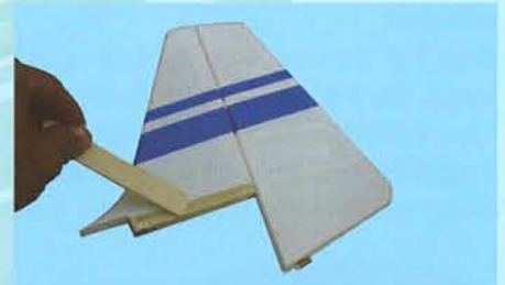
8C- Apply sufficient 30 minute epoxy to the exposed wood in the vertical stabilizer
