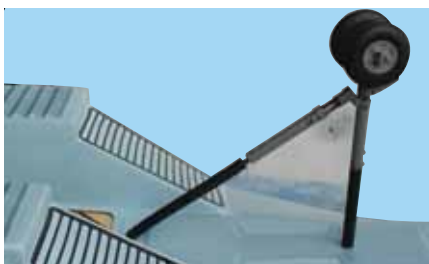
9C - Insert the front nose gear oleo strut and the support strut.
