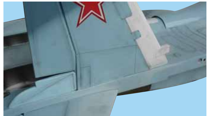
6C - Trial fit the vertical stabilizer in its slot
