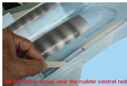
6E - Apply plenty of epoxy into the fuselage slot for the vertical stabilizer
