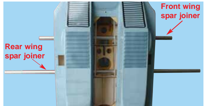
1C - Insert the wing joiners into the fuselage
