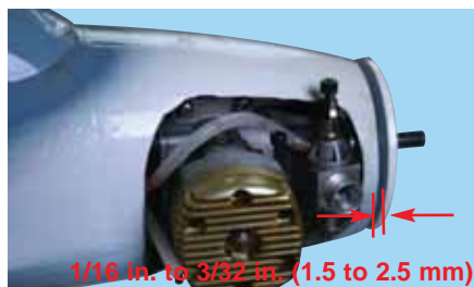
12B - Allow for gap between the spinner back plate and the fuselage
