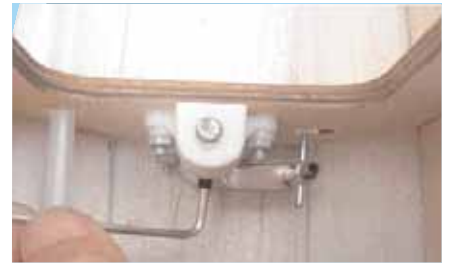
9G - After re-inserting the nose gear oleo strut, align and tighten the steering arm set screw.
