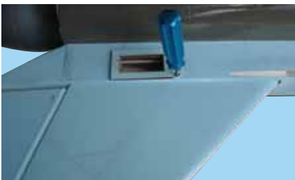
5F - Use 3mm steel rod or screw driver to align the rudder hole guide
