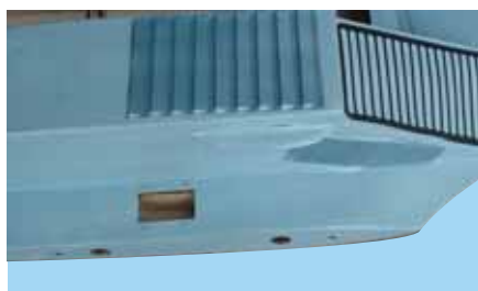
8B - Main landing gear location on the fuselage (left side)
