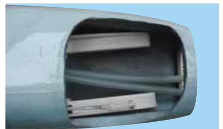
10D - Fuel tank installed into the fuselage after adding external fuel lines from tank forward to engine area
