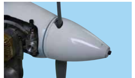
15D - Install the spinner cone using the retaining bolt. Ensure the retaining bolt is tight and secure
