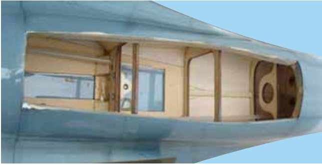
11A - Remove the cockpit and instrument panel from the fuselage
