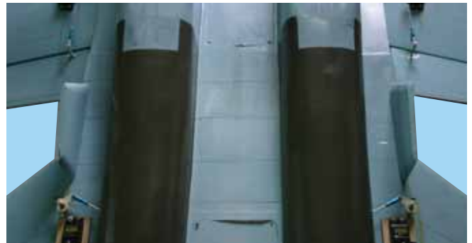
28D - Ventral fins attached to the fuselage straight and square.
