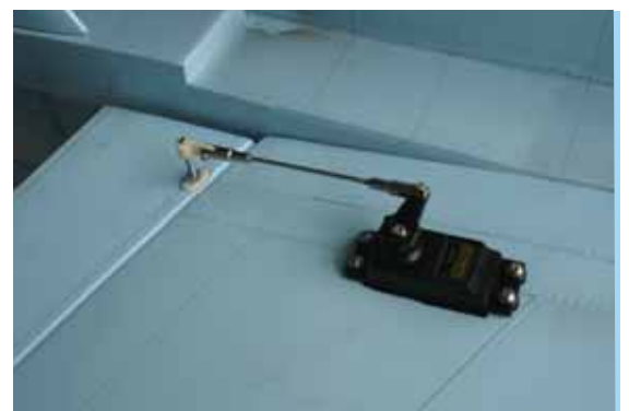
3C- Aileron control rod installed
