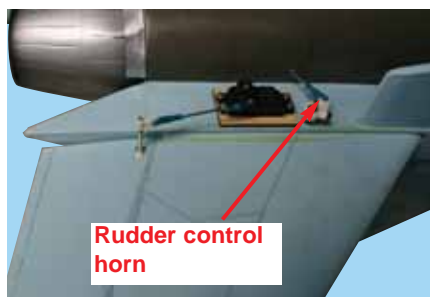
19A - Connect the 2 rudder control rods to the rudder control horns.
