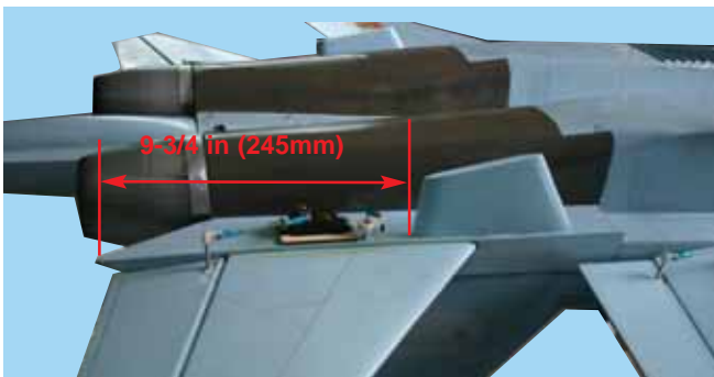
28C - Use 30 minute epoxy to glue the left ventral fin to the fuselage
