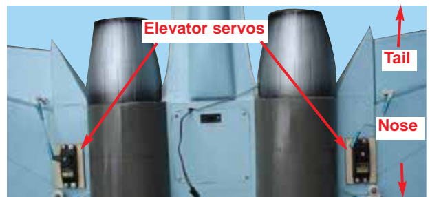
18B - Connecting the elevators to the servos
