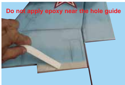
6D - Apply sufficient epoxy to both sides of the exposed wood
