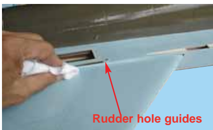
5E - Wipe off the excess epoxy
