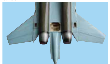
5G - After installation of both horizontal stabilizers
