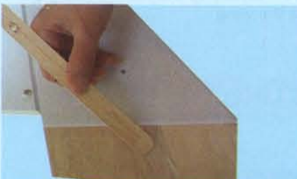
6C - Apply sufficient epoxy to the exposed wood area on both sides and into the fuselage slot
