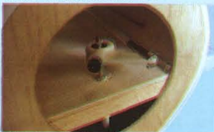
19C - Connect the clevis to the control horn and then tighten the set screw securely
