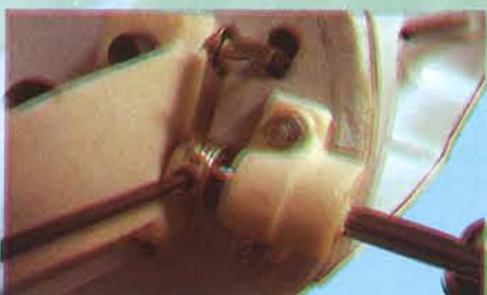
9C - Secure the steering arm to the nose gear wire by tightening the set screw
