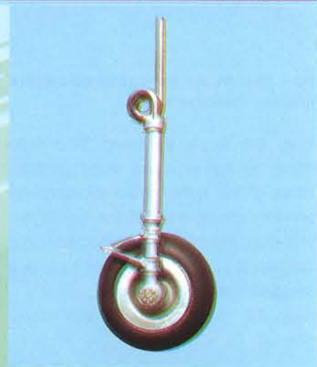
9A - Nose gear assembly
