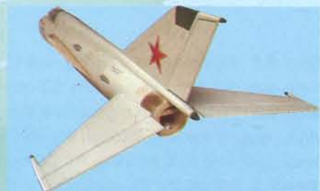
6F - Vertical and horizontal stabilizer installed
