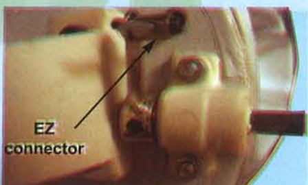
9D - Secure the EZ-connector to the nose gear push rod by tightening the set screw
