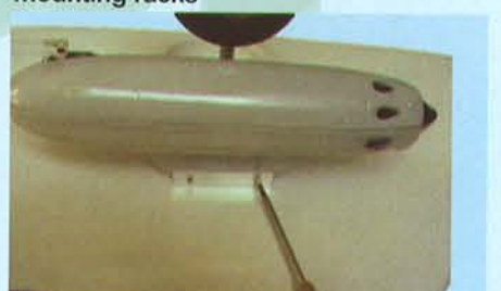
29D - Mount the dummy tanks to the aluminum racks on the wings
