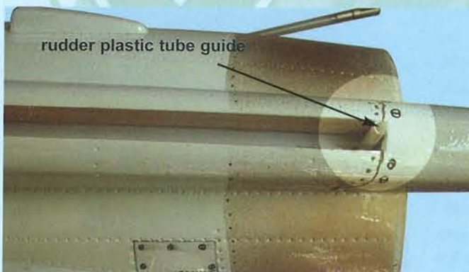
5B - Vertical slot with pre-installed rudder plastic tube guide
