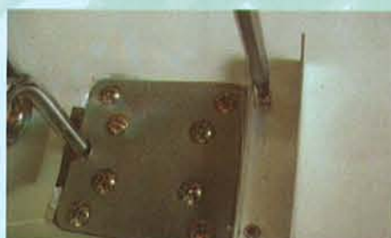
29C - Mount the aluminum racks to the wings.
