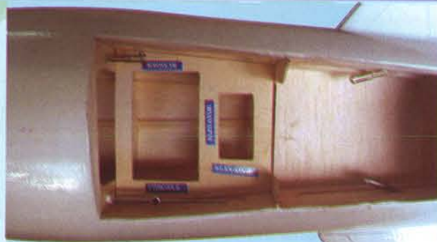
17A - Location of elevator (2), rudder and throttle 9
