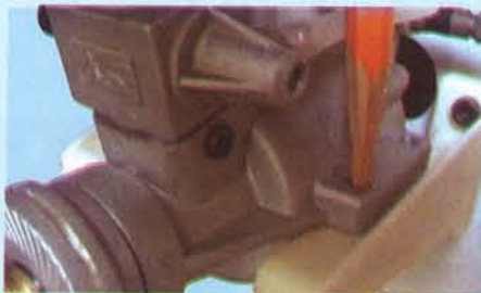
12C - Mark the location of the engine mounting holes
