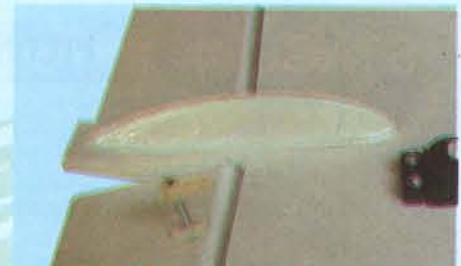
2C - Mount the aileron servo into the wing
