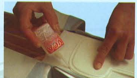
28C - Glue the nose gear cavity cover into place using CA glue
