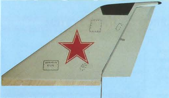
4B - Vertical stabilizer with pre-installed rudder
