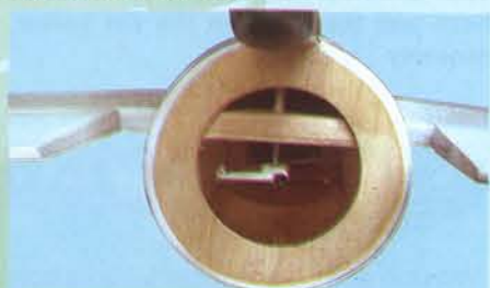
16D - Rudder control horn installed
