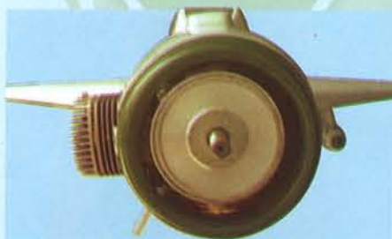
15B - Install the spinner backing plate
