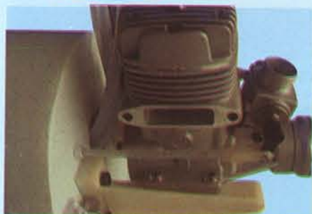
13A - Connect the clevis to the engine throttle arm
