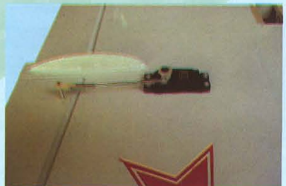
3C - Aileron control rod installed
