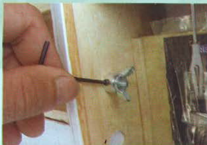
1.7 Tighten the hex-bolt on collar to secure the attachment
