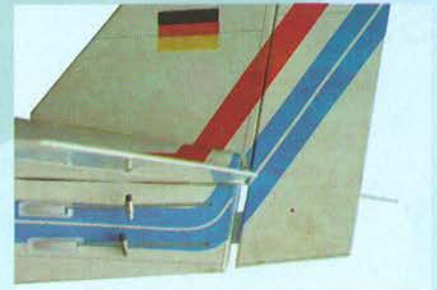
12.3 Insert the pre-installed hinge to the rudder
