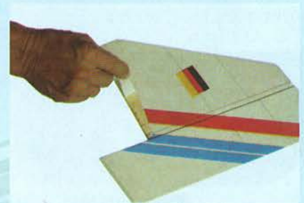
11.3 Remove covering from both sides
