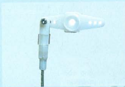
20.2 Install EZ connector to the servo arm
