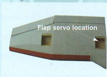
4.2 Flap servo in each wing
