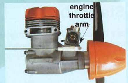
23.2 Throttle control rod connected to the engine throttle arm
