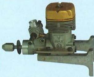
17.5 Fitting the engine to the engine mount
