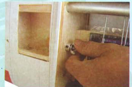
1.6 Insert the aluminum collar then tighten the wing bolt
