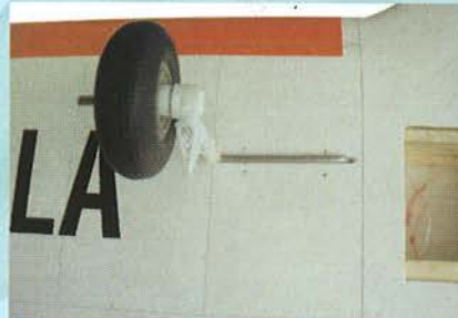
15.4 Main landing gear in place
