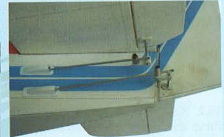
22.2 Connecting the rudder pushrod to the rudder control horn
