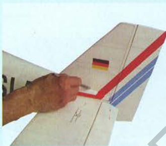
11.1 Mark both sides of the vertical stabilizer
