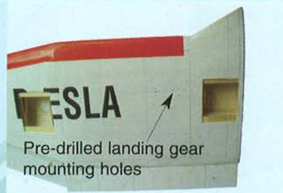
15.2 Main landing gear location
