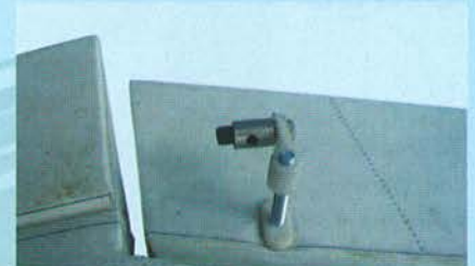
2.5 Install aileron control horn
