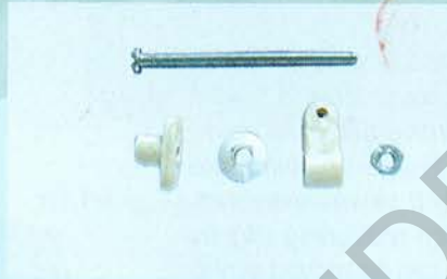
3.2 Aileron control horn assembly
