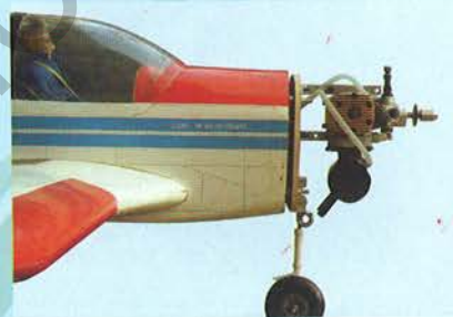
17.12 Power module mounted to the fuselage (side view)
