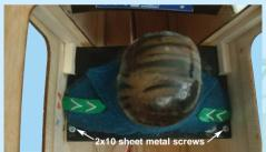
27D- Install the dummy pilot onto the rails and secure into place with two 2x10 [mm] screws
