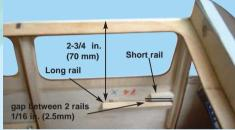
27C- Glue the rails to the left side of the fuselage
