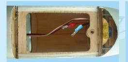
28B- Battery compartment as seen from bottom of fuse-lage
