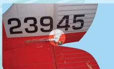
18A-Hold the rudder at neutral (not left, not right). Rotate the clevis to adjust the overall length. Then use the clevis screw to attach the clevis to the control horn. The clevis screw requires a 5/64 in. (2mm) hole. Secure the screw with thread lock
