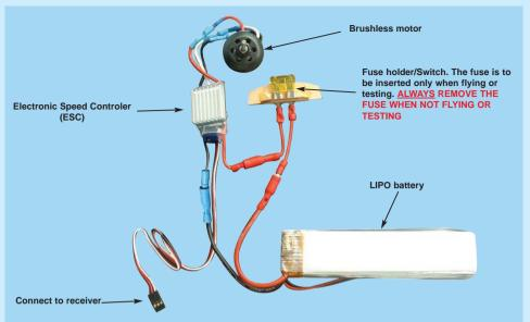
12M- Typical wiring diagram of brushless motor system
