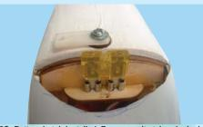
28C- Battery hatch installed. Fuse security tab unlocked
