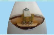
28D- Battery hatch installed. Fuse security tab in place
