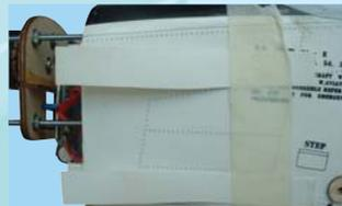
13B- Card stock strips overlying the cowl mounting tabs on the left side of the fuselage
