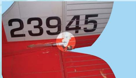
18A- Hold the rudder at neutral (not left, not right). Rotate the clevis to adjust the overall length. Then use the clevis screw to attach the clevis to the control horn. The clevis screw requires a 5/64 in. (2mm) hole. Secure the screw with thread lock
