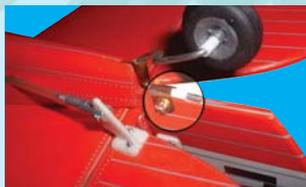
11C- Attach the Rudder Flange to the rudder using a 3x8 bolt as shown
