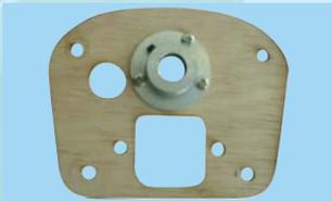
12C- Securely mount the aluminum motor backing plate to the firewall using 3 nut, bolt & washer sets provided. Tighten the nuts securely and apply thread locker such as Pacer Z-42 (Blue)
