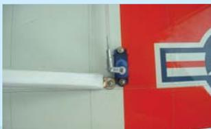
26E- Strut attached to the wing
