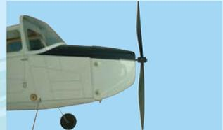
13G- With the **BATTERY & FUSE REMOVED** securely install the propeller
