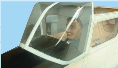
27E- Dummy pilot after installation
