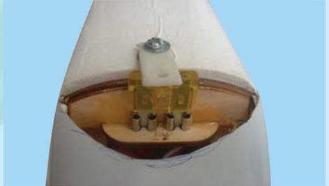
28D- Battery hatch installed. Fuse security tab in place
