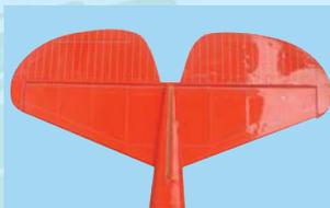
6A- Trial fit the horizontal stabilizer in its slot
