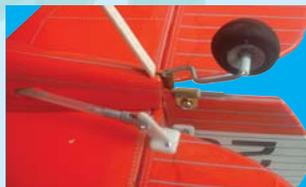
11D- Apply 30 Minute Epoxy into the slot to secure the anchor flange
