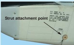
26D- Strut attachment point on the right side of the fuselage
