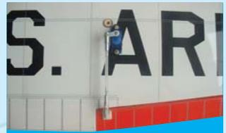
4C- Connect the aileron control rod between the servo arm and the control horn
