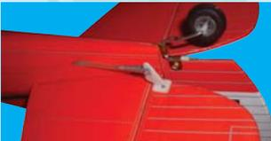
17A- Elevator control horn shown in position
