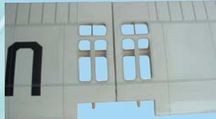
**2B-** Align the two wing panels and slowly close the gap until the wing root ends are firmly in contact with each other
