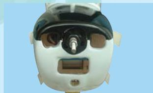
13D- Position the cowl over the mounting tabs. Note the strips are outboard. Align & center with respect to the motor shaft
