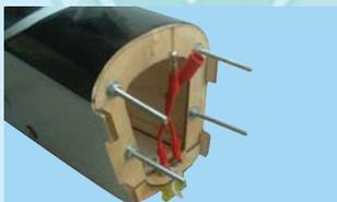
12J- Install four 3x50 [mm] bolt sets (supplied). Bolt-washer-former-washer-nut (front). Tighten the nuts securely & apply thread locker
