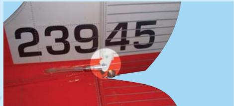
14D- Rudder control horn location
