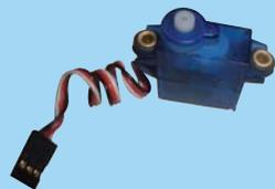
**3A-** Prepare the servos by fitting the rubber grommets & ferrules supplied with your servos
