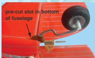
11B- Insert the anchor flange into the slot in the bottom of the fuselage
