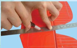
7D- Cutting inside the lines. **Do NOT cut the wood**
