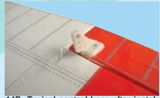
14B- Typical control horn after installation
