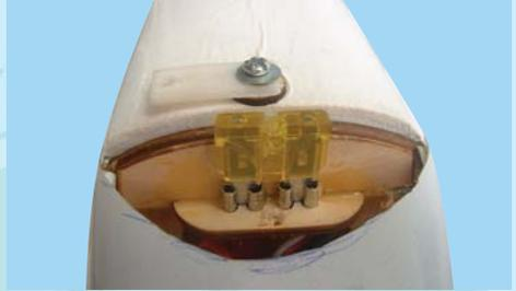
28C- Battery hatch installed. Fuse security tab unlocked
