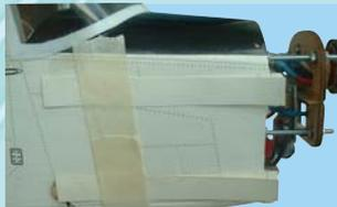
13A- Card stock strips overlying the cowl mounting tabs on the right side of the fuselage
