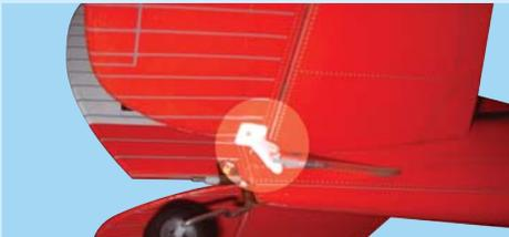
14C- Elevator control horn location
