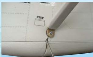
26F- Strut attached to the fuselage
