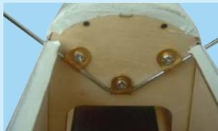
10C- Use three 3x8 [mm] bolts to secure the main landing gear to the fuselage
