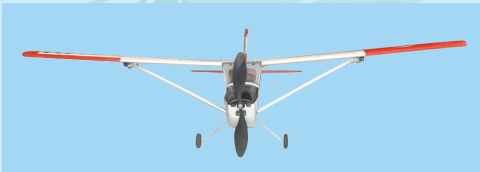
26G- Left & right struts installed to model
