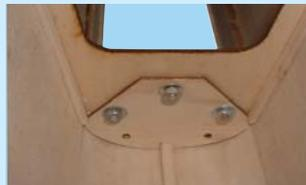
10D- Use washers and firmly tighten the nuts to secure the landing gear
