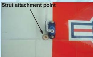
26A- Strut attachment point on the underside of the right wing
