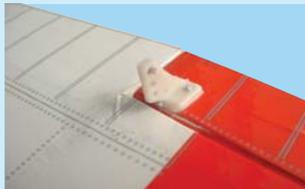
4B- Aileron control horn after installation.
