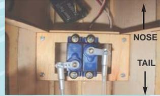
16A- Center the servo control surface and then connect the control rods to the servos using the clevises as shown
