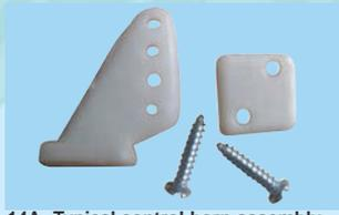
14A- Typical control horn assembly
