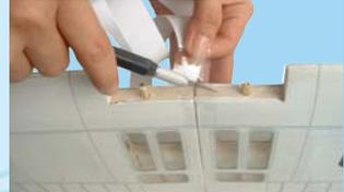
**2F-** Continue back around to the bottom of the wing & overlap the tape where you started. Trim off excess tape
