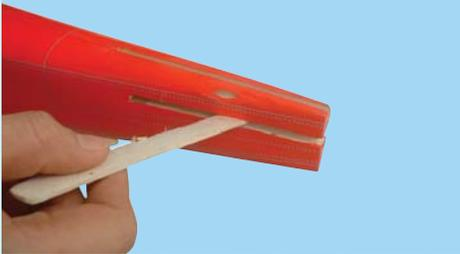
7H- Apply plenty of 30 minute epoxy into the horizontal slot
