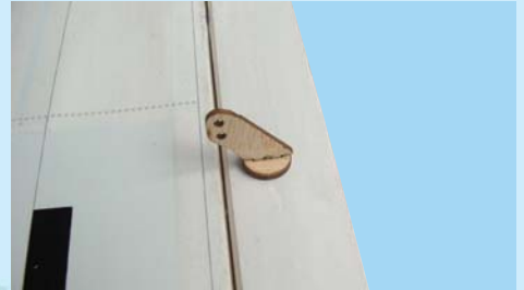
1D- The holes in the control horn must align with the hinge line
