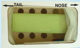
25F- Using foam to secure the battery
