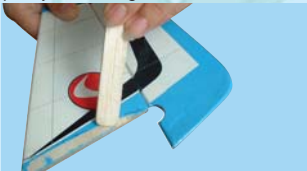
7E- Apply plenty of 30 minute epoxy
