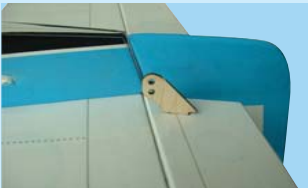
13C- Using 30 minute epoxy install the elevator control horn into the pre-cut slot
