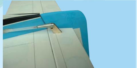
16B- Hold the elevator at neutral (not up, not down). Rotate the clevis to adjust the overall length. Then use the clevis screw to attach the clevis to the control horn. The clevis screw requires a 5/64 in. (2mm) hole. Secure the screw with thread lock
