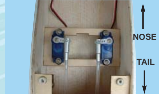
15A- Center the servo control surface and then connect the control rods to the servos using the clevises as shown
