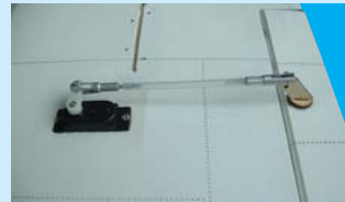
3C- Connect the aileron control rod between the servo arm and the control horn
