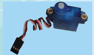
2A- Prepare the servos by fitting the rubber grommets & ferrules supplied with your servos
