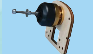
11C- Install the motor to the firewall using 4 bolts (3x10mm) & washer sets provided. Place washer on bolt and insert bolt through back of firewall & screw into tapped holes in motor mounting plate. Secure bolts with medium thread locker
