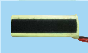
25D- Glue Velcro (hook) to the battery
