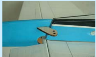
13E- Using 30 minute epoxy install the rudder control horn into the pre-cut slot
