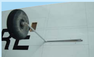
9C- Insert the pre-bent main landing gear into the wing
