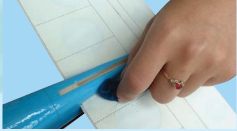
6K- Wipe off excess 30 minute epoxy
