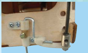
10C- Use four 2x10 [mm] screws to install the nose gear assembly. Then insert the control rod into the EZ connector and tighten the set screw
