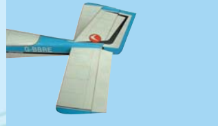
7A- Trial fit the vertical stabilizer into the fuselage slot
