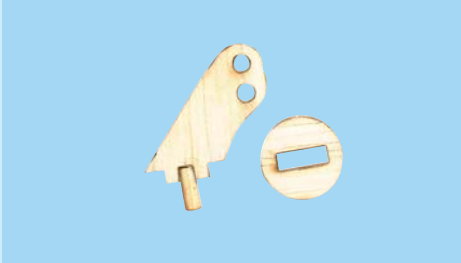
1A- Aileron control horn
