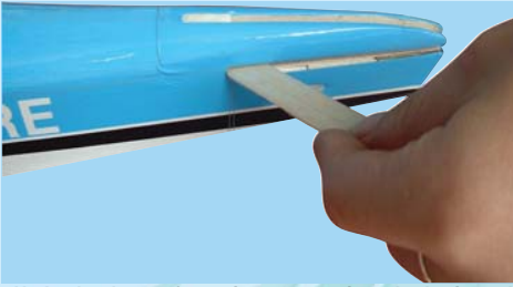
6H- Apply plenty of 30 minute epoxy into the horizontal slot
