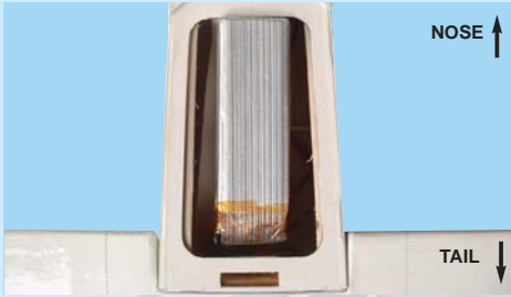
26C- Battery installed with fuse removed
