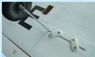
9D- Use two straps and four 10x2 [mm] screws to mount each main landing gear assembly
