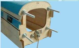
11J- Install four 3x30 [mm] bolt sets (supplied). Bolt-washer-former-washer-nut (front). Tighten the nuts securely & apply thread locker
