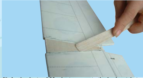
6I- Apply plenty of 30 minute epoxy to the horizontal stabilizer
