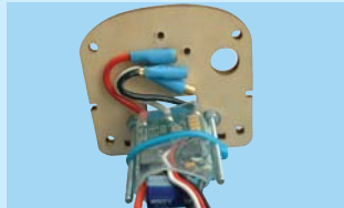
11E- Secure the Electronic Speed Control to the restraining bolts using a tie wrap as shown
