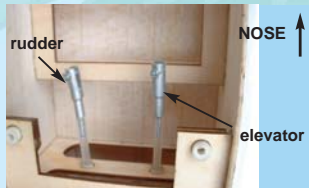
14C- Note the orientation and positions of the elevator and rudder control rods
