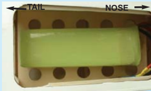
25E- Install the battery using the Velcro
