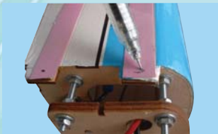
12C- Mark the strip with a dot at the center of each cowl mounting tab
