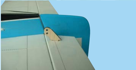
16A- Elevator control horn shown in position
