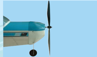
12G- With the BATTERY & FUSE REMOVED securely install the propeller
