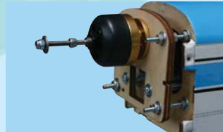
11L- Place four 3 mm washers on the bolts & then position the assembled power module. Secure in place with four more 3 mm washers & nuts. Tighten snugly
