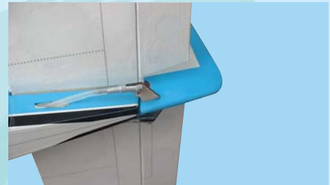
17A- Hold the rudder at neutral (not left, not right). Rotate the clevis to adjust the overall length. Then use the clevis screw to attach the clevis to the control horn. The clevis screw requires a 5/64 in. (2mm) hole. Secure the screw with thread lock
