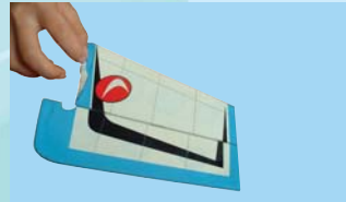
7D- Remove covering from both sides
