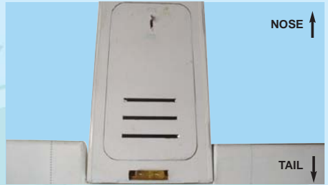
26D- Battery hatch and fuse installed
