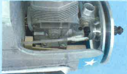
14A- Connect the clevis to the engine throttle arm
