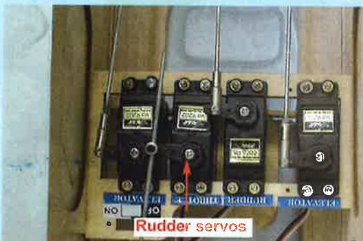
20A- Connecting the rudder control rod to the servo
