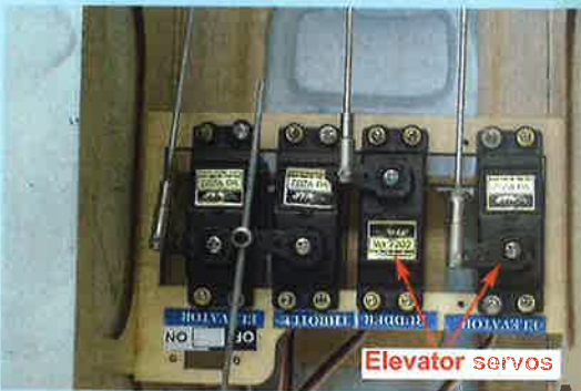
19A- Connecting the elevator control rod to the servos
