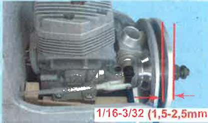
13A- Allow for gap between the spinner back plate and the fuselage
