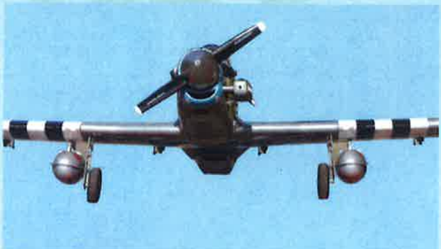
32C- 2 dummy fuel tanks mounted to the plane
