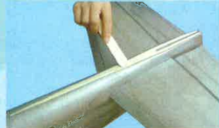
8C- Apply sufficient epoxy to the exposed wood area in the fuselage
