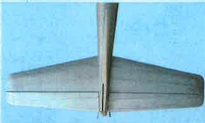
7G- Press both horizontal stabilizers until it hit the fuselage
