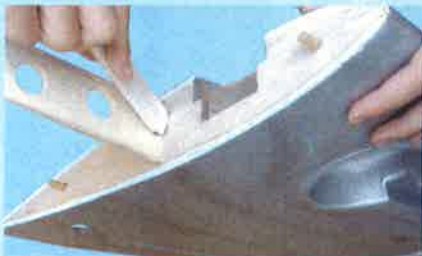
2A- Apply plenty of 30 minute epoxy glue to all surface
