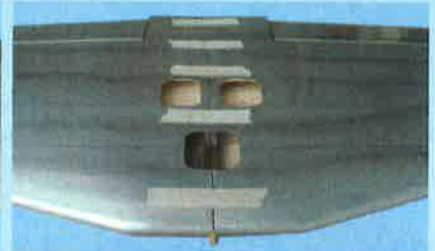
2C- Use low tack masking tape to hold tightly together
