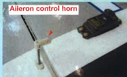
5B- Aileron control horn and servo
