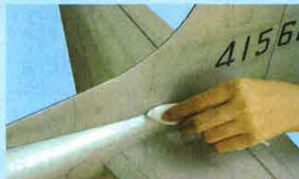
8E- Wipe off the excess epoxy
