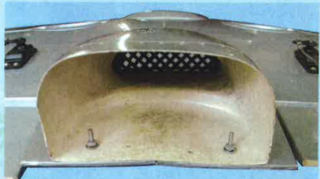
30B- Air scoop installed to the wing
