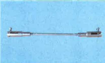
5A- Aileron control rod assembly
