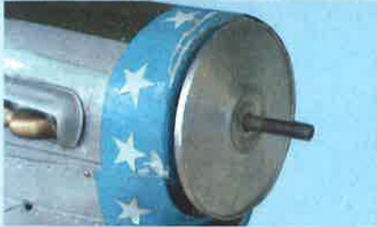
16B- Install the spinner backing plate
