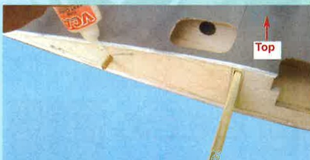
1C - Apply CA glue to secure dowels into their places
