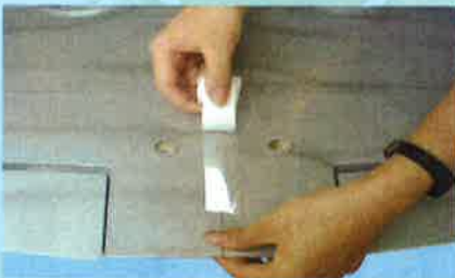
3A- Apply tape over the joint starting here on the bottom wing
