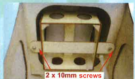
12C- Fuel tank assembly in position
