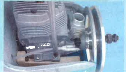
13D- Use four 4 x 25mm sheet metal screws to mount the engine.
