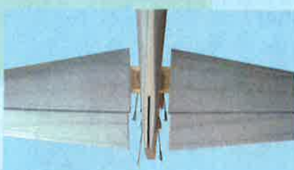
7F slowly press both horizontal stabilizers to the fuselage
