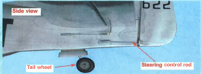
10B- Pre-installed tail wheel assembly with steering rod connected to the rudder
