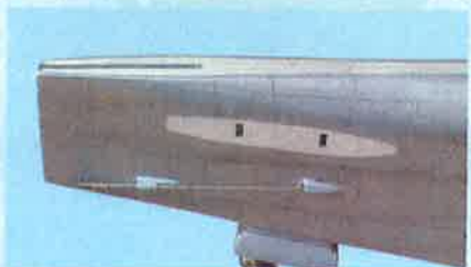
6A- The fuselage slots for the vertical & horizontal stabilizer
