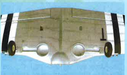
9C- Both main landing gear mounted to the wing
