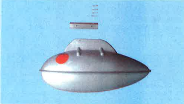
32A- Dummy fuel tank with mounting hardware
