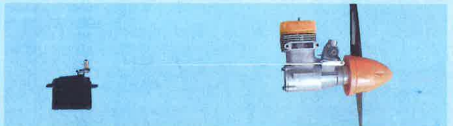
14B- Connect the servo arm to the engine throttle arm using the throttle control rod
