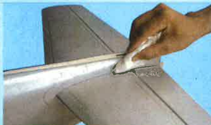
7H- Wipe off the excess epoxy
