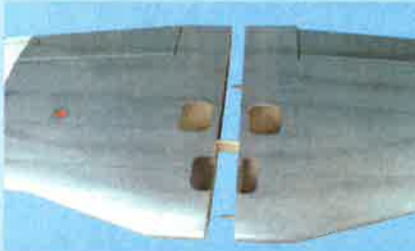
2B- Align the two wing panels and slowly close the gap until the wing root end are firmly in contact with each other
