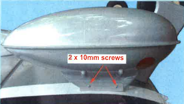
32C- Mount the dummy fuel tank to the rail
