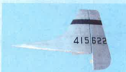
6B- Vertical stabilizer with pre- installed rudder
