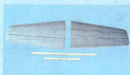
6C- Horizontal stabilizer with pre- installed elevator and 2 elevator joiner
