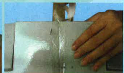
3C- Continue over the top of the wing and trim off the excess tape
