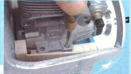
13B- Mark the location of the engine mounting holes
