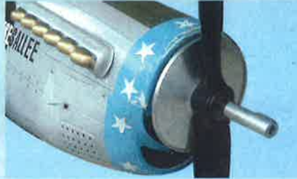
16C- Install the propeller, the prop washer and the prop nut
