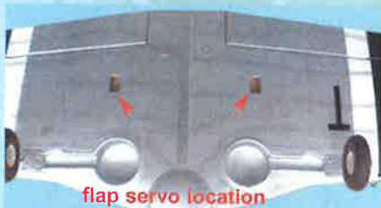
28A- Flaps and flap servo cavity locations
