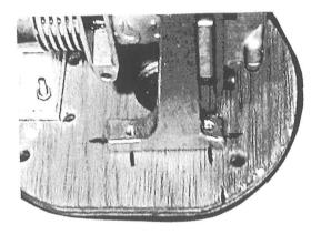
**5.1.4** Use the pencil to mark the engine mount hole(as shown),once you have the hole location, drill the hole with 6mm (1/4 in) drill bit
