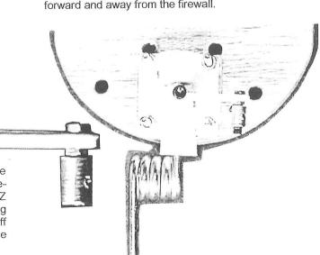
3.4.2 Install the steerable nose gear using the nose gear wire, the nose gear steering arm, the pre-installed nose gear block and the pre-installed EZ connector that will connect the nose gear steering arm to your steering servo. To do this...first back off the steering arm set screw. Now put the end of the steering wire to the pre-installed EZ connector.
