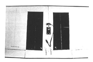
**2.2.3** Screw the servo into place with the screws and grommets.
