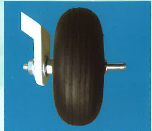
18.2 Install the axle and wheel to the main gear
