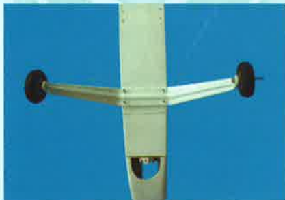
19.3 Use 4 sheet metal screws (5 x 35mm) to mount the main landing gear onto the fuselage
