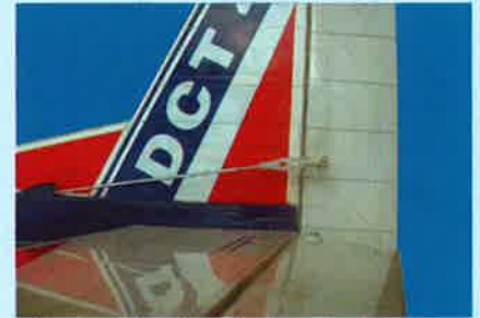
30.2 Connecting the rudder pushrod to the rudder control horn
