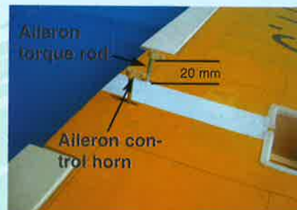
7.3 Aileron torque rod with control horn
