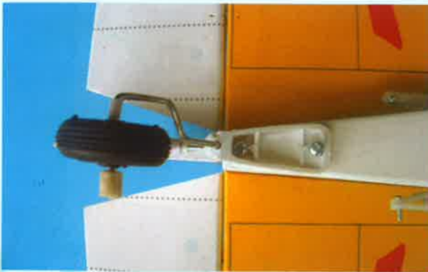
19.6 Screw the tail wheel assembly to the fuselage
