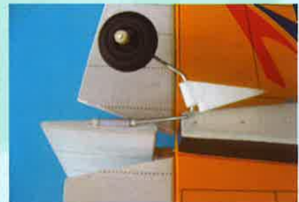
19.5 Insert the tail wheel steering wire into the steering guide tube
