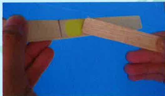
2.1 Apply epoxy to one end of wing joiner
