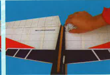
13.4 Wipe off excess epoxy
