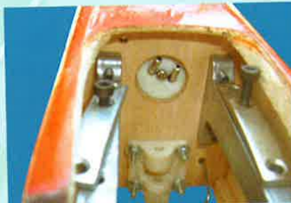
22.2 Use a 4mm socket ball wrench or Allen Key to remove the 4 black machine screws that work with the clamping plates on the metal engine mount that has been pre-installed into your Apache III
