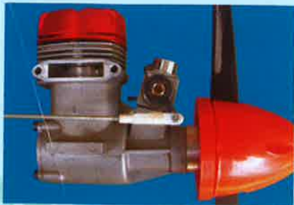
23.1 Clevis attached to engine throttle arm
