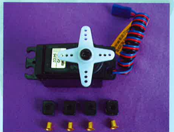
5.1 Prepare the servos by fitting the rubber grommets & ferrules supplied with your radio
