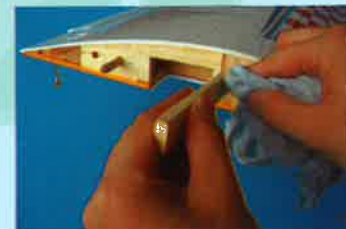
2.4 Wipe off the excess epoxy
