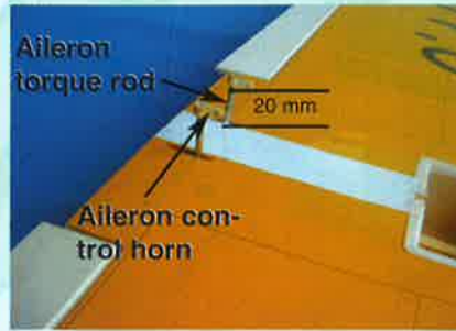
8.2 Aileron torque rod with control horn
