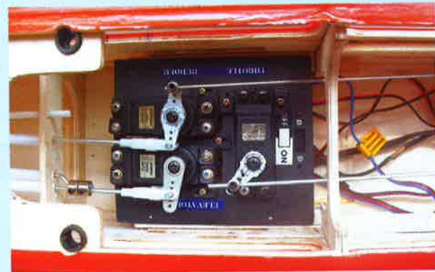
27.3 Throttle, elevator and rudder servos connected to their pushrods
