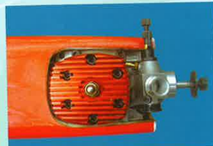
22.3 Remove the muffler, position the engine on the engine mount and confirm that the fuel tank metal tubes clear back of the engine. Trial fit the engine temporarily into plates. Tighten the screws only enough to tack the engine into place
