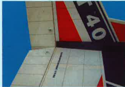
30.1 Rudder control horn installed and shown in position
