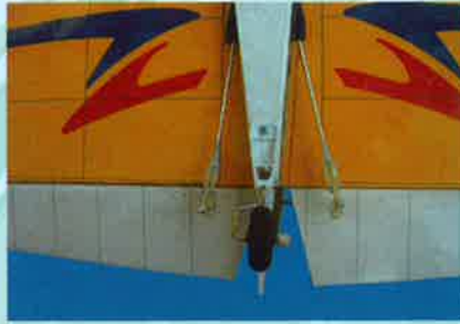
29.2 Connecting the elevator pushrods to the control horns
