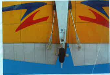
26.5 Elevator control horn connected to the control rod
