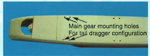
19.2 Turn over the fuselage to locate the 4 pre-drilled main landing gear mounting holes (as shown)
