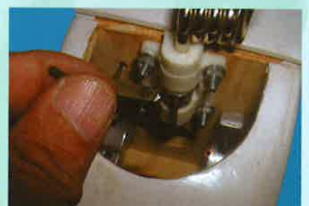
20.8 Now tighten the nosegear steering arm
