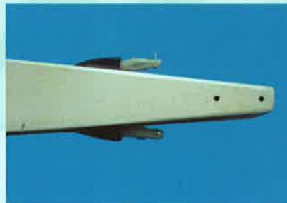
19.4 Turn over the fuselage to locate the 2 pre-drilled tail wheel mounting holes (as shown)
