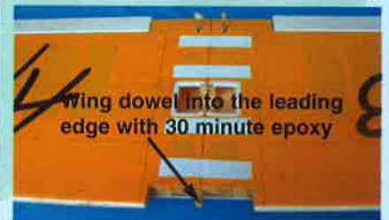
3.4 Use tape to hold tightly together also install the wing dowel
