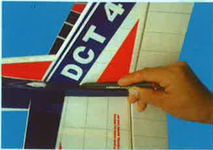
15.1 Mark both sides of the vertical stabilizer
