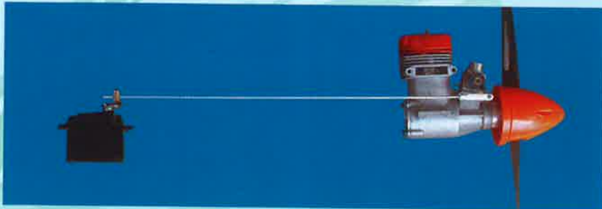
23.2 Throttle control rod connected to the engine throttle arm and to the servo arm
