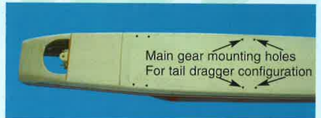
20.2 Turn over the fuselage to locate the 4 pre-drilled main landing gear mounting holes (as shown)
