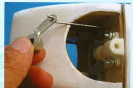
20.5 Put the end of the pre-installed Z-bend wire through the hole in the steering arm
