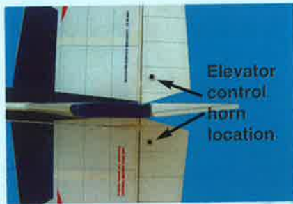
26.3 Elevator control horn location
