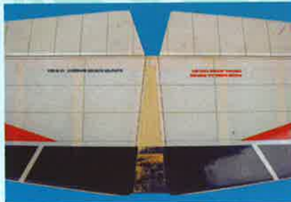
12.3 Removed covering from top surface
