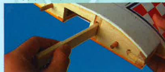
2.2 Carefully insert the joiner... Also the dowel guide
