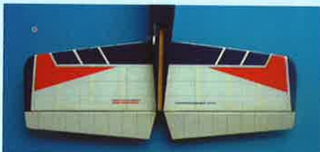
10.1 Trial fit the horizontal stabilizer in its slot
