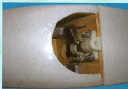
20.7 Holding the nosegear steering arm in place, slide the nosegear into the nylon mount, passing through the steering arm.
