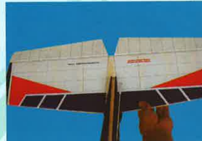
13.3 Slide the horizontal stabilizer in place
