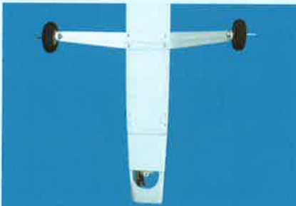
20.3 Use 4 sheet metal screws (5 x 35mm) to mount the main landing gear onto the fuselage
