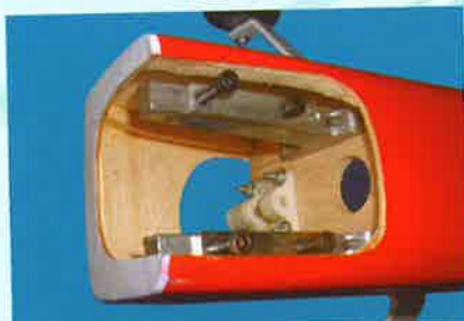
22.1 Engine mount pre-installed into the fuselage
