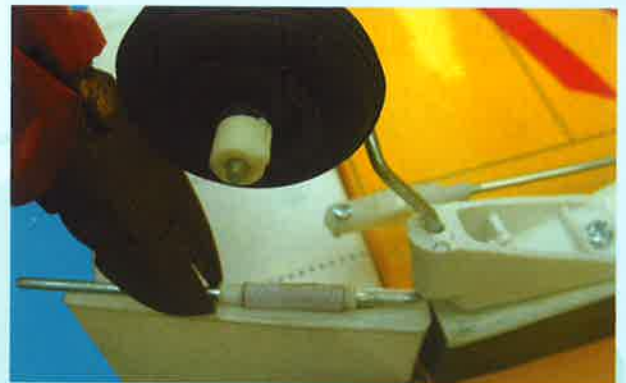
19.7 Trim off the excess tail wheel steering wire
